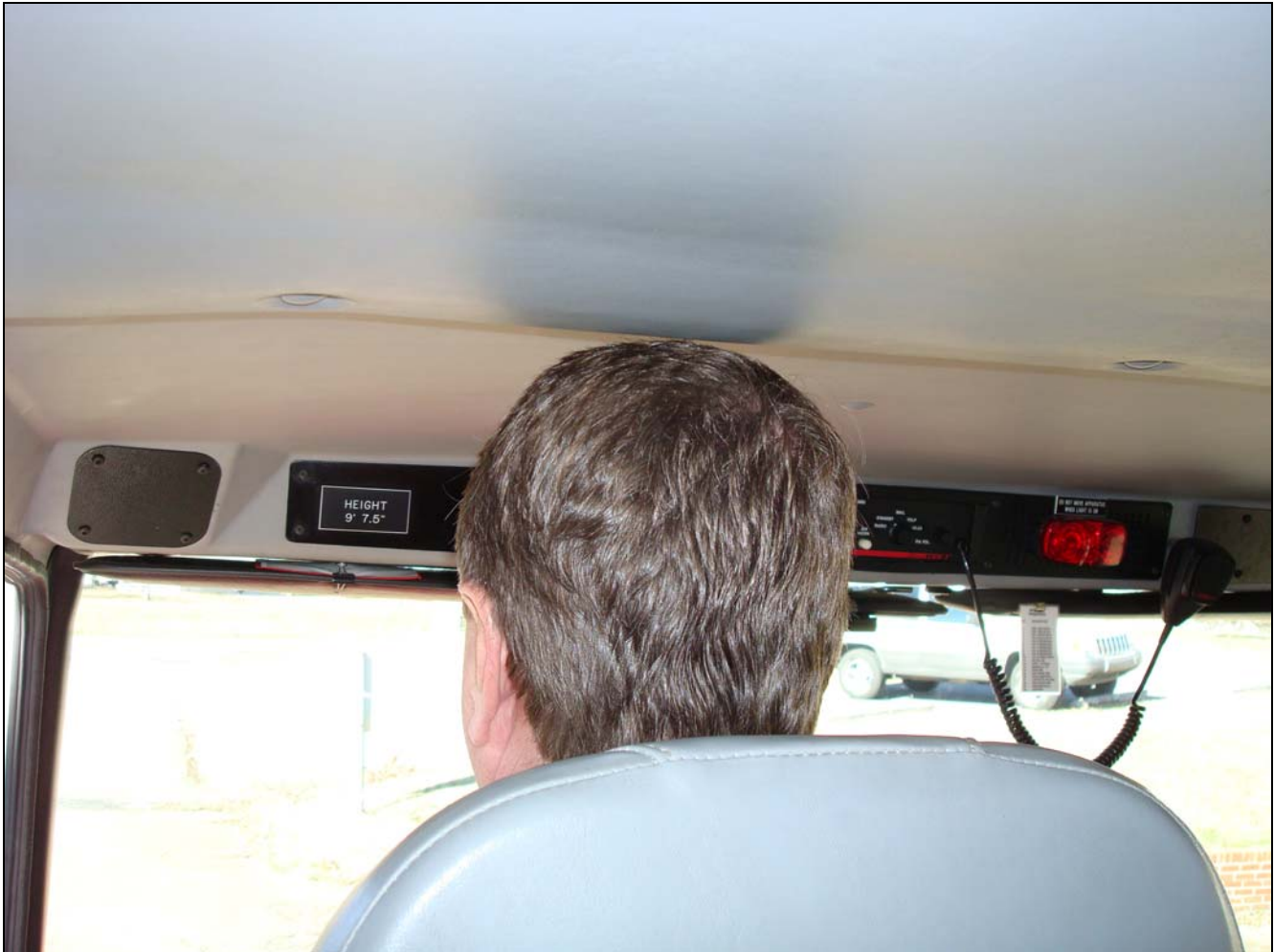
Photo 6. Similar fire truck showing clearance between head and cab ceiling. Note: Seat is raised and subject is close to the height of the victim. (Photo by NIOSH.)
