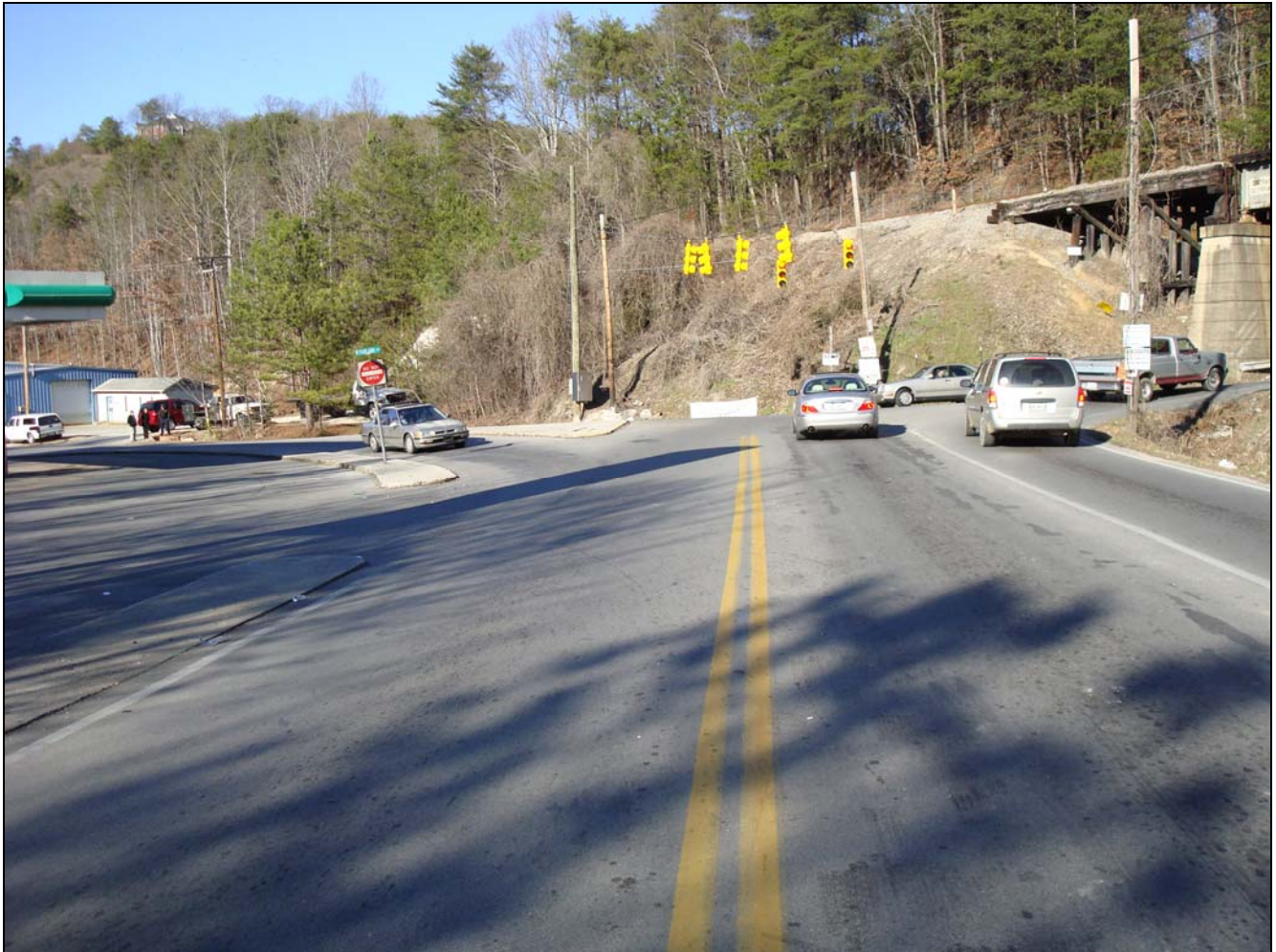
Photo 2. Intersection approach. Note the railroad trestle on the right, restricting the view of oncoming traffic. (Photo by NIOSH.)
