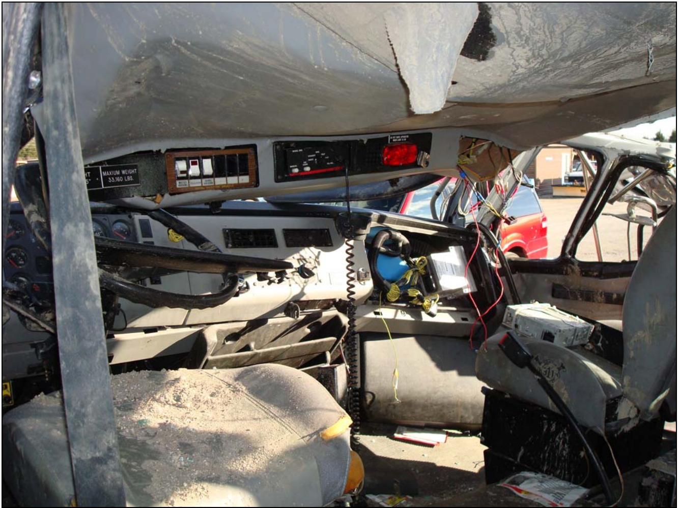
Photo 5. Roof of cab intruding into driver's area. Note: Seat back was removed during extrication. (Photo by NIOSH.)
