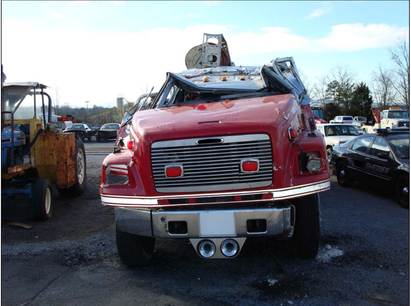
Photo 4. Cab roof intrusion into driver and passenger compartment. (Photo by NIOSH.)
