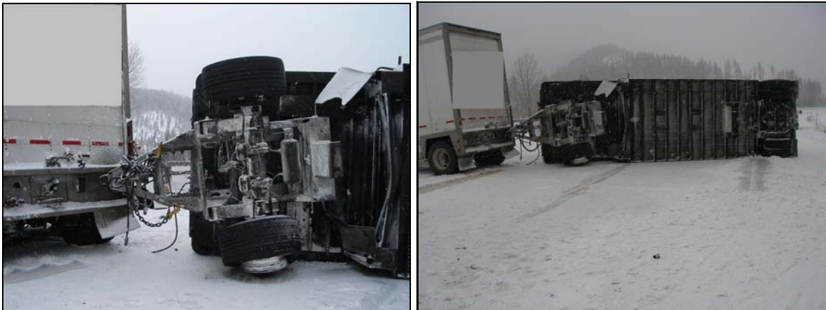
Photo 1. Dolly used to pull second trailer in tandem. (Photo courtesy of State Highway Patrol)
