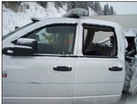
Photo 4. Showing virtually no damage to the passenger compartment. (Photo courtesy of fire department)
