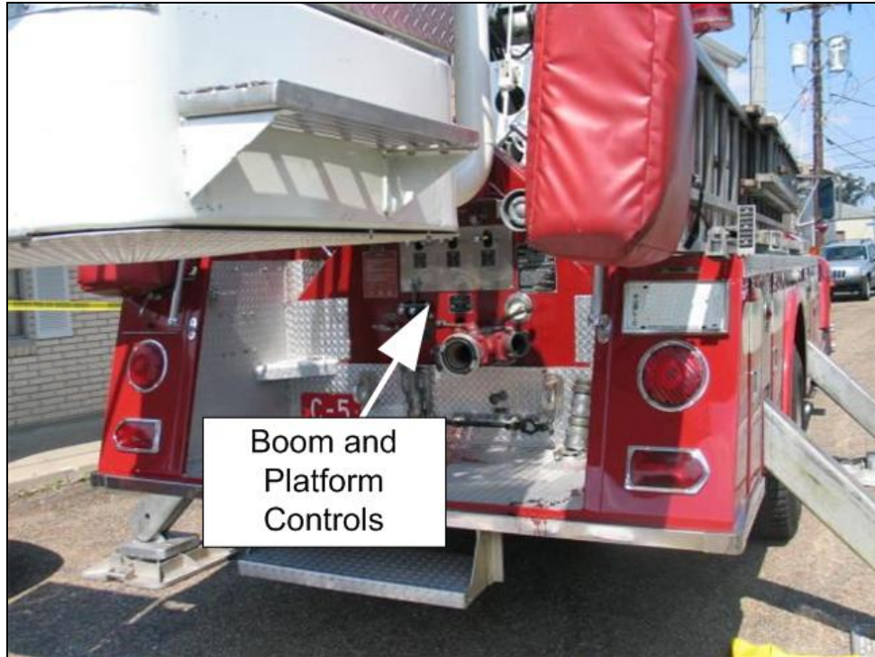
Photo 2: Tailboard controls underneath boom in cradled position.
