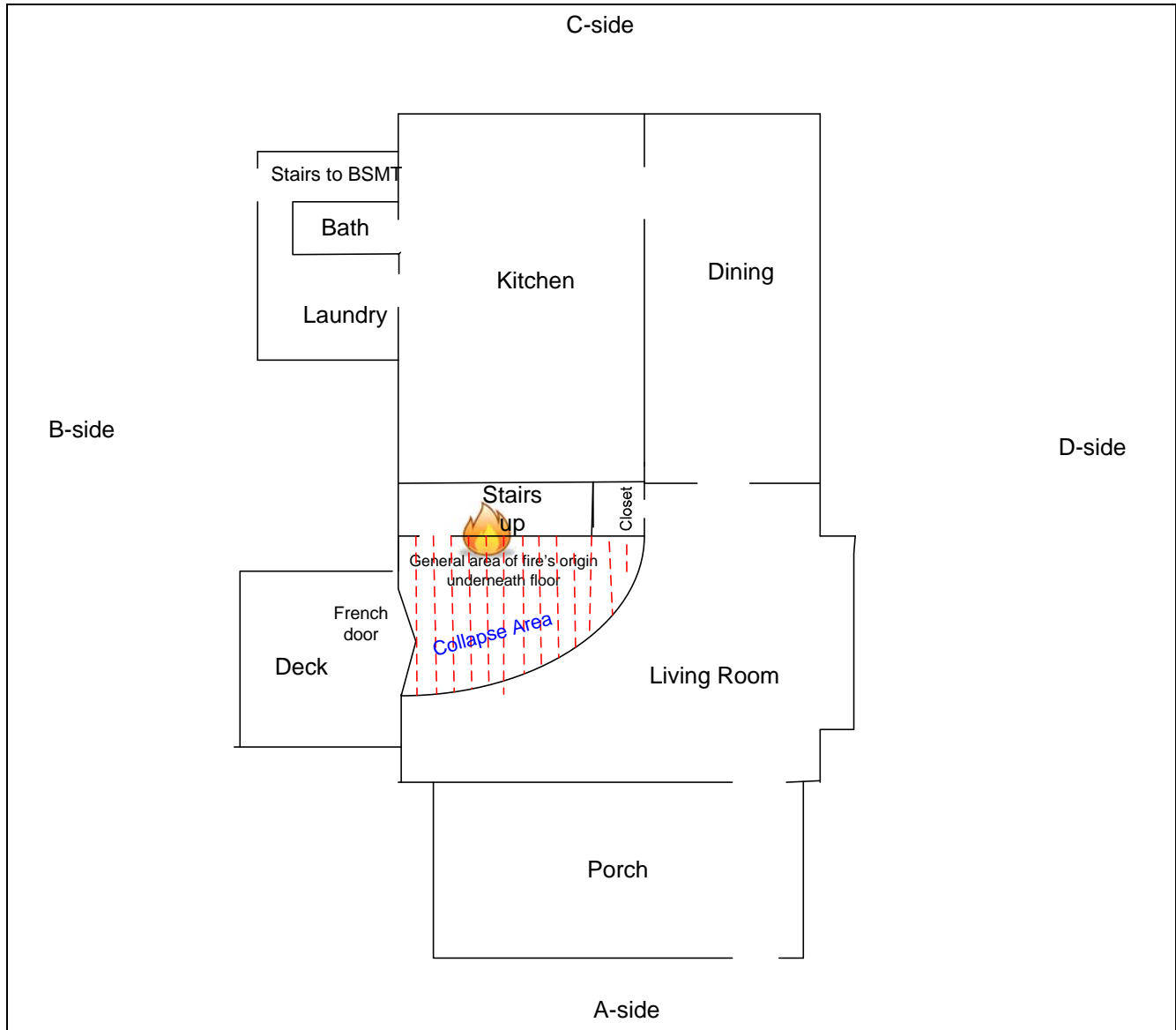
Diagram 3. Depicts the fire structure's first floor layout, collapsed area, and approximate location of the fire's origin.
