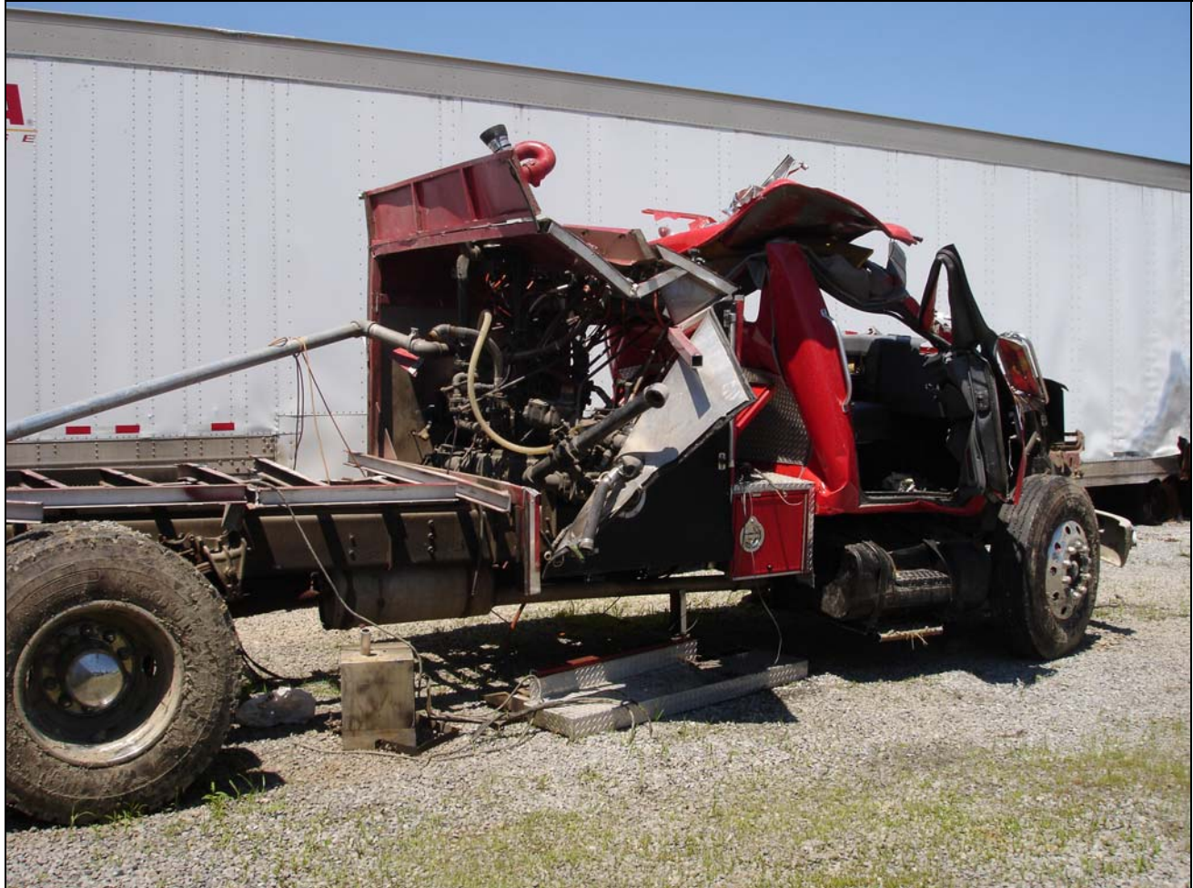
Photo 2. Side of apparatus after incident. (NIOSH photo.)
