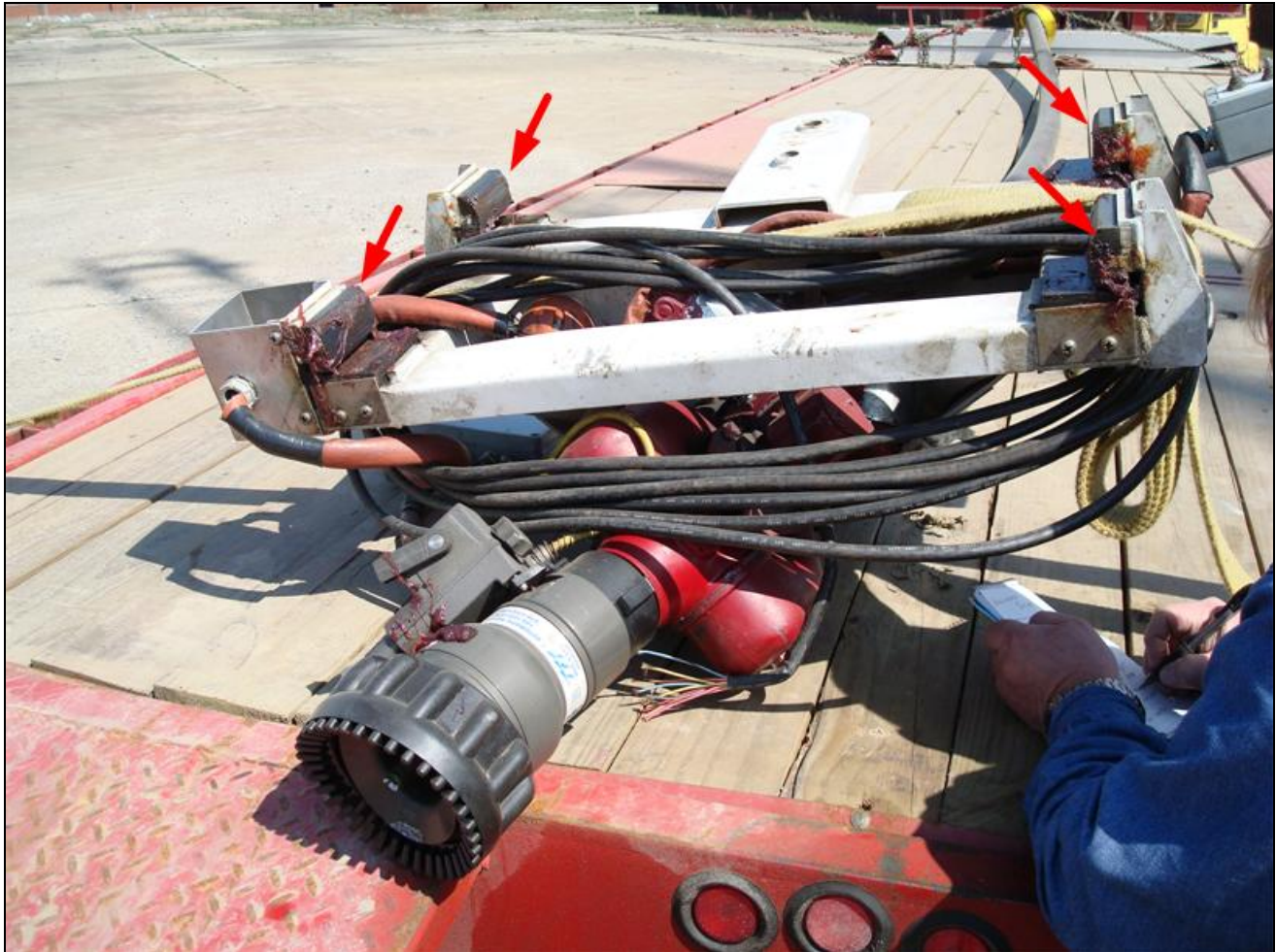
Photo 2. Waterway that “launched” during incident. Arrows depict Nylatron ® pads that are greased to aid movement as the ladder extends and retracts. (NIOSH photo.)
