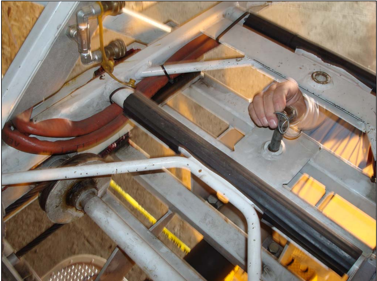
Photo 4. Aerial ladder involved in the incident. Photo shows pin being inserted into the rear or lower hole. This is the pin position for rescue operations (water monitor pinned to second section of ladder – this hole is the rear or lower of the two). (NIOSH photo.)
