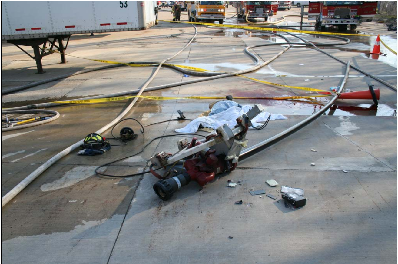
Photo 6. Waterway is in foreground near the location where it struck the victim. Photo shows distance the waterway traveled after it was “launched.” Note ladder truck L-289 at top right. (Photo courtesy of Matt Skrekla.)
