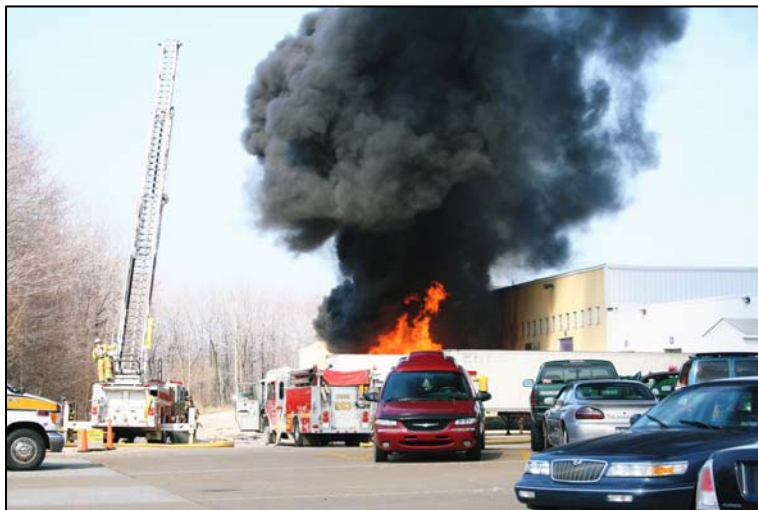
Photo 1. Aerial ladder being raised into position for master stream operation.
