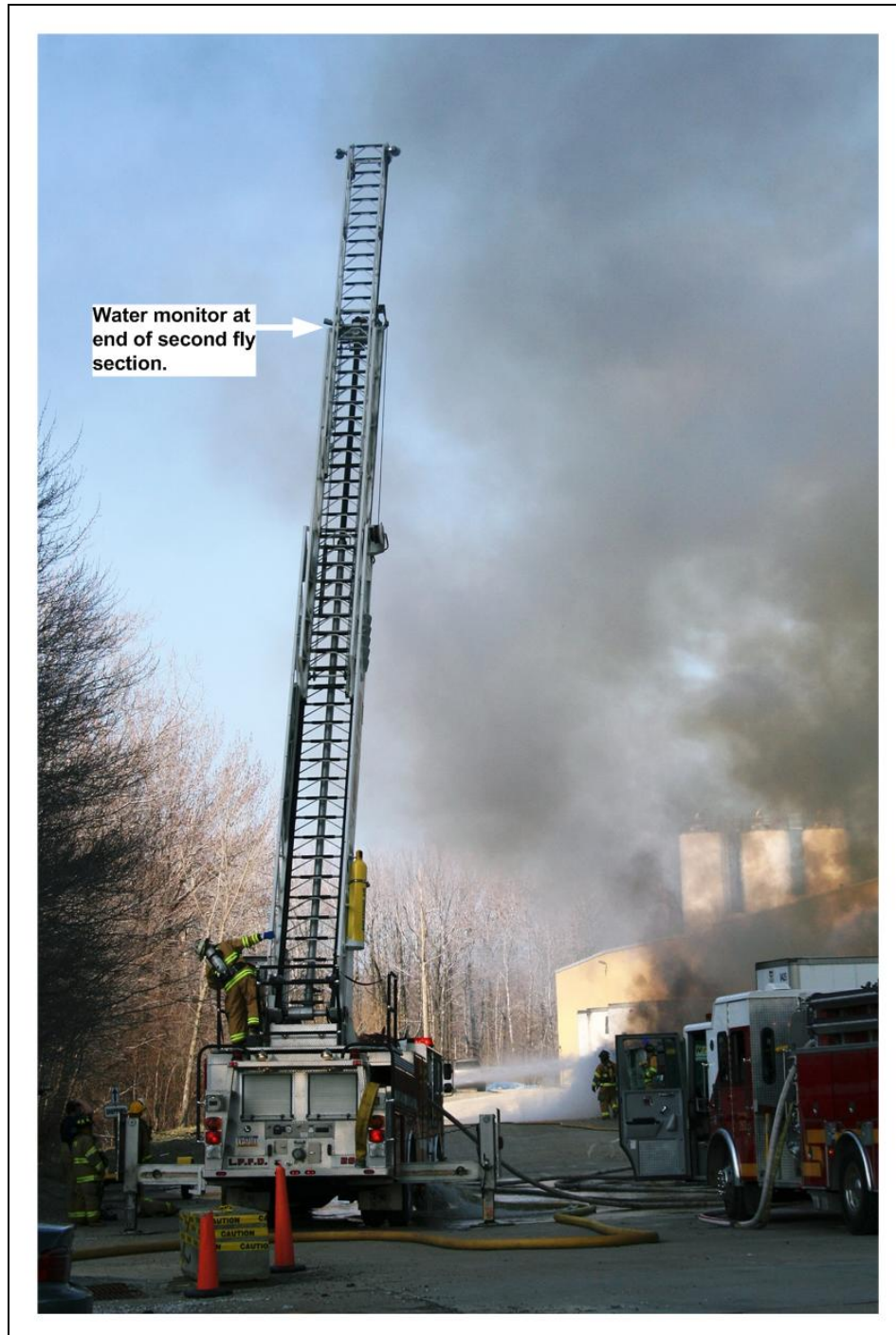
Photo 5. Photo taken just seconds before fatal launch. Note the water monitor is still in the rescue position. ( Photo courtesy of Matt Skrekla.)
