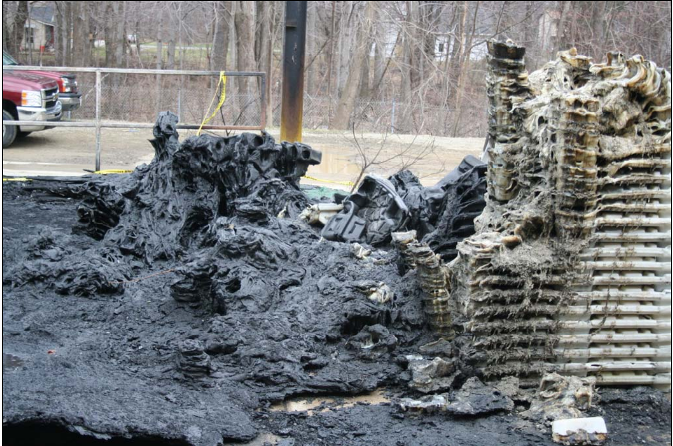
Photo 8. Plastic pallets and other plastic materials on the loading dock immediately after fire. (Photo courtesy of Matt Skrekla)
