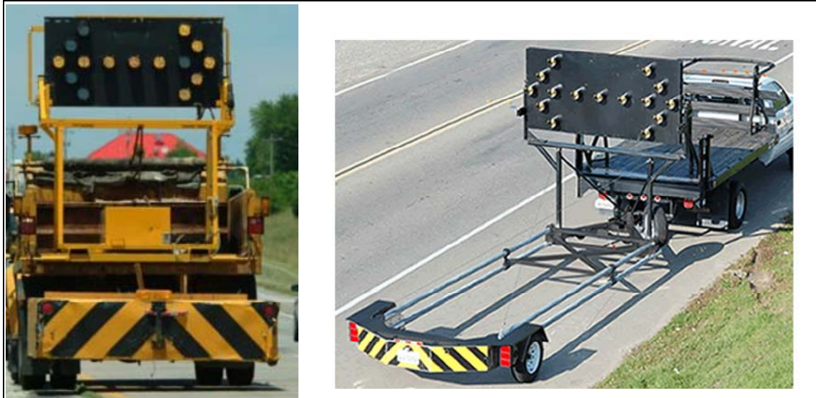
Photo 4. Examples of truck mounted attenuators.
