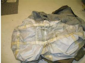
Photo 3. The repaired crotch area of the turnout pants shell, and inverted liner with diminished thermal integrity due to age and use.
