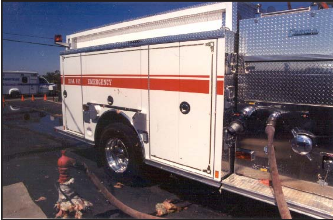
Photo 1. Illustrates the engine's passenger side discharge panel. It also depicts the fill line connected to the #4 discharge and water holding tank's hydrant.
