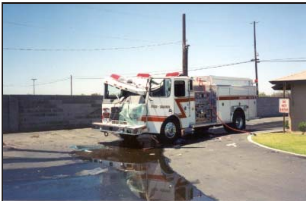
Photo 4. Depicts the point of impact by the holding tank on the cab of the engine.
