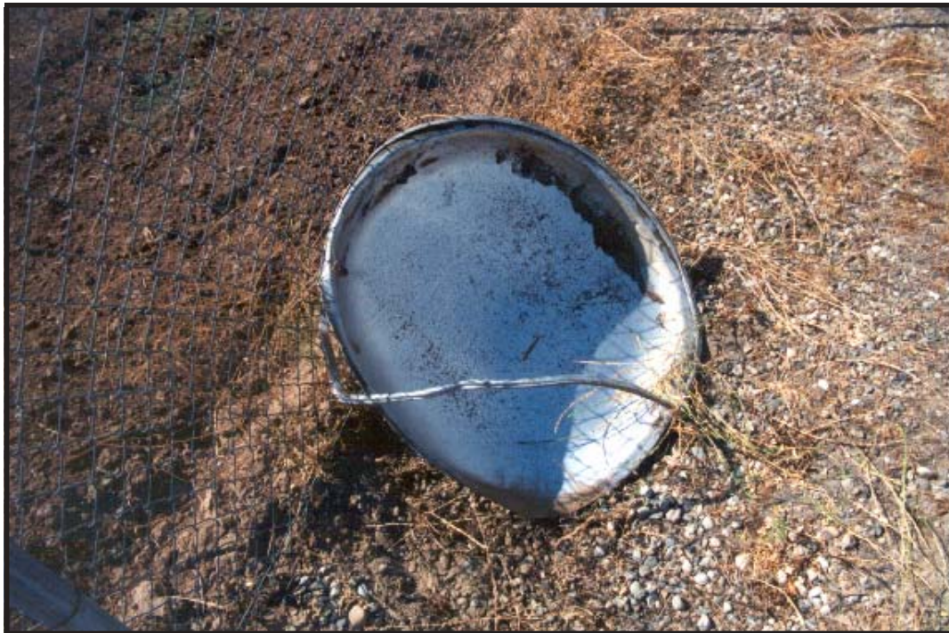
Photo 5. Illustrates that the holding tank failed near the bottom seam.
