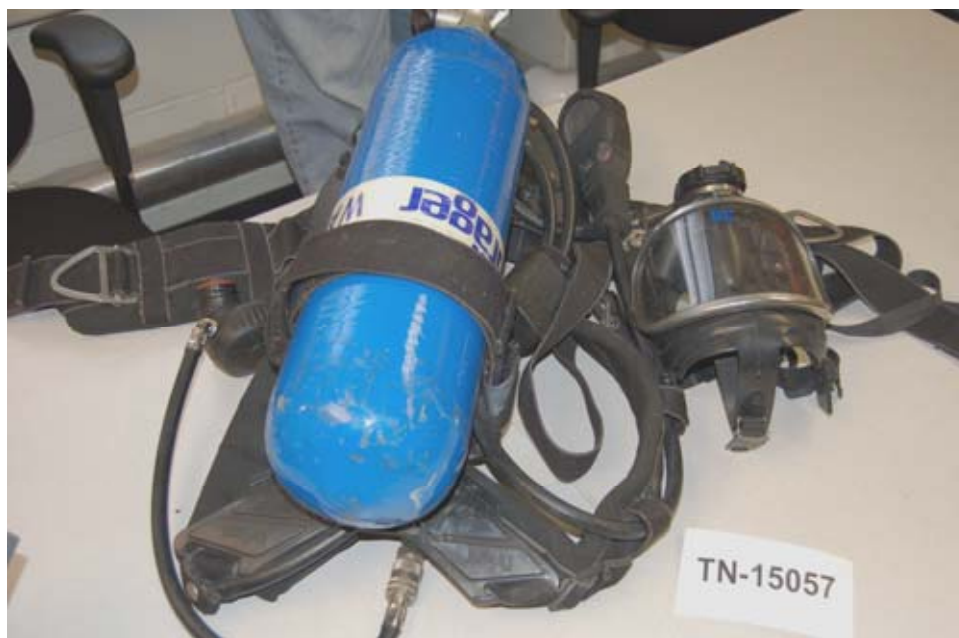
Figure 2 – SCBA Ready for Inspection
