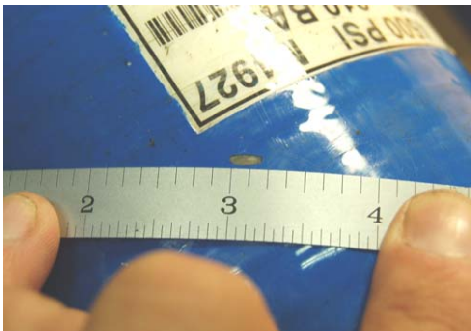
Figure 24 – Gouge in Cylinder Sidewall
