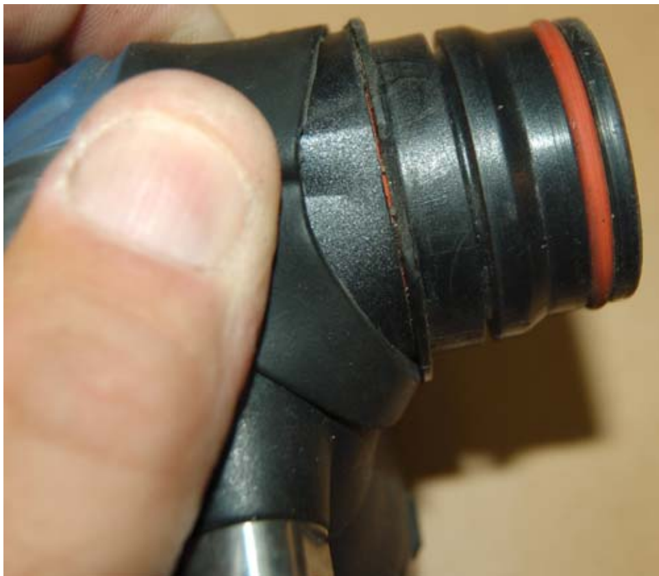
Figure 10 – Separation of Barrel from Lung Demand Valve Housing
