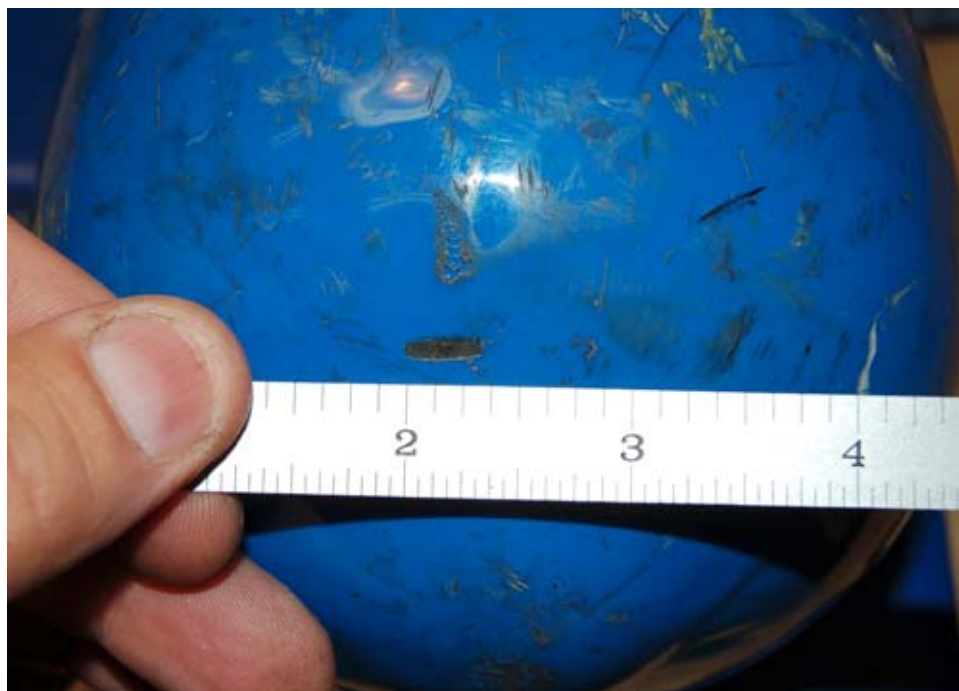
Figure 23 – Gouge in Cylinder Dome
