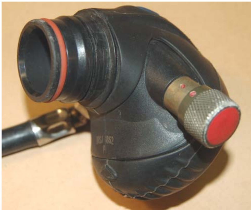
Figure 8 – Side View of Lung Demand Valve
