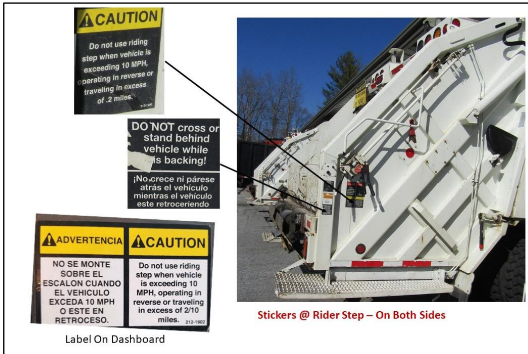
Passenger side rear label with locations on refuse truck. Photo courtesy of NC OSHA
