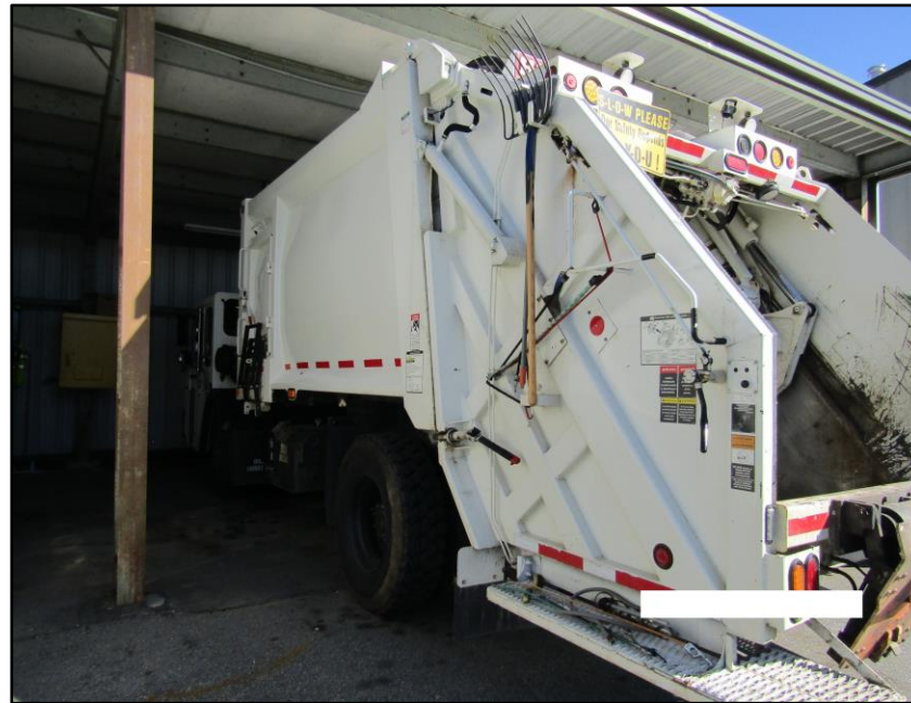
2016 Crane Carrier model LETZ-30 truck chassis with a 2016 Heil model PT1000 refuse collection attachment. Photo courtesy of NC OSHA
