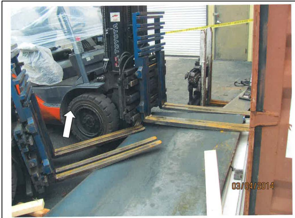
Photo 1. Incident scene, pallet with material on the ground; arrow indicates forklift involved. (Photo courtesy of TOSHA.)
