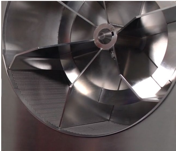
Figure 3 – Impeller and milling screen
