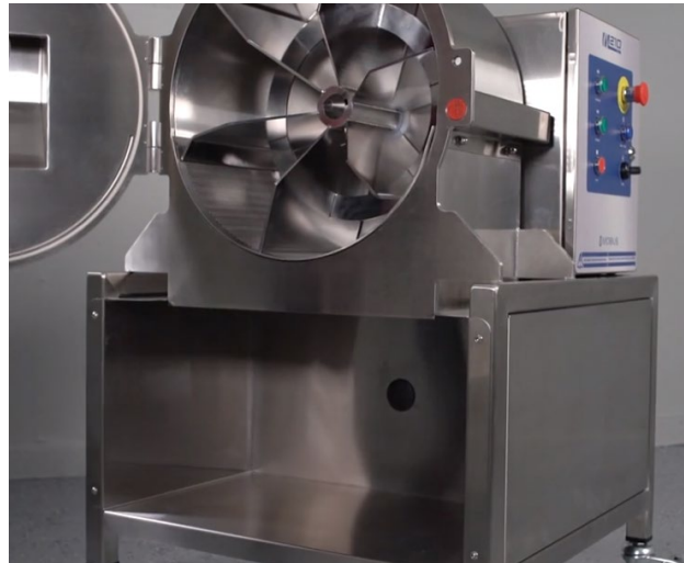
Figure 4 – Impeller and collection area, bin removed
