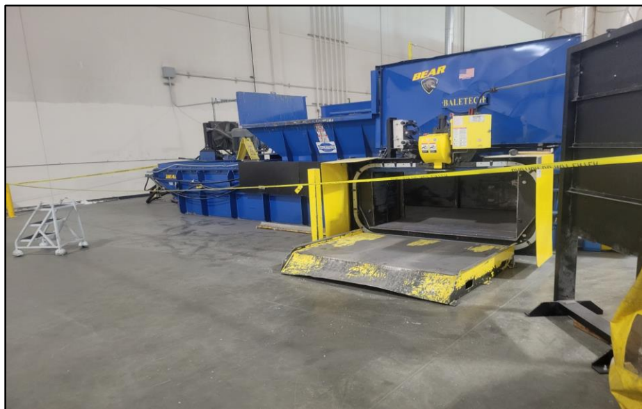
Exhibit 2. The location where the finished bale is expelled. Photo by CA/FACE program.
