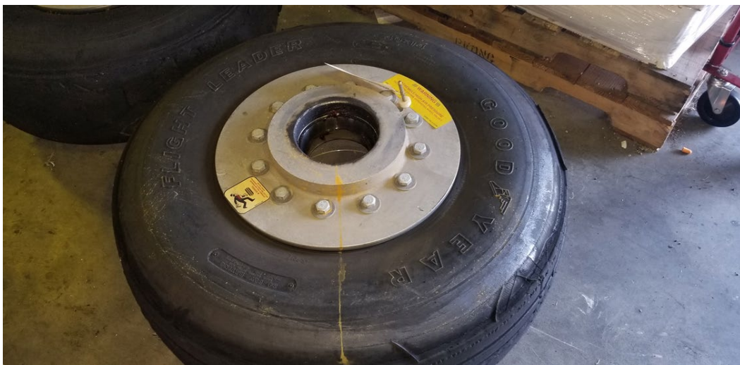
Exhibit 3. Tire and wheel assembly similar to the one involved in the incident, showing the 12-bolt pattern holding the wheel assembly together.
