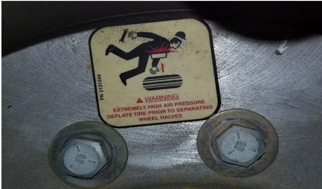
Exhibit 6. Second warning sticker placed on all tire/wheel assemblies used on passenger boarding bridges.
