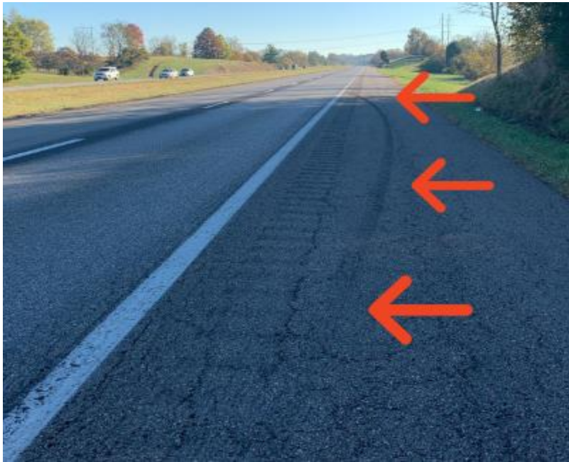
Photo 1. Photo depicting the path traveled as the dump truck crossed the median and struck the earth embankment. Yaw marks were produced by the passengers' side front steer axle tire which resulted from the driver taking evasive action. Photo property of KY FACE.
