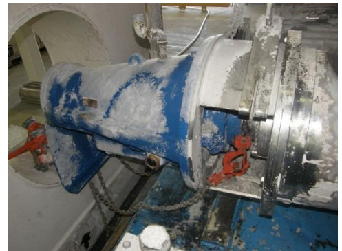
Photo 4 “Come-along” lever pullers attached to recirculation pump.
