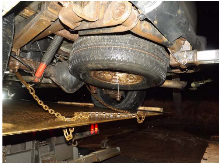
Photo 2. Picture of cable lowered but tire not released from safety retaining system while pickup truck on tow truck flatbed.
