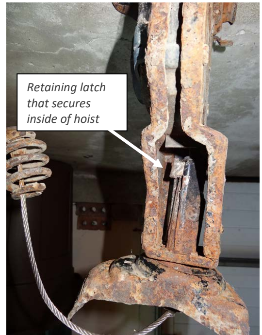
Photo 6. Spare tire hoist system from a similar make and model year of pickup truck involved in incident.
