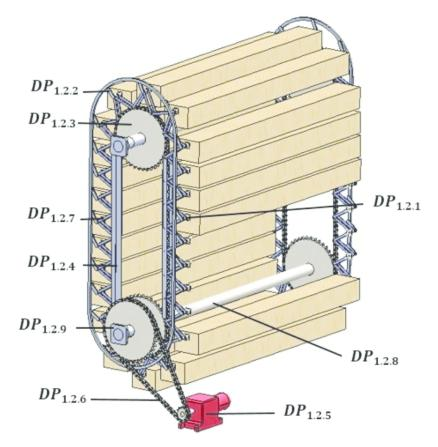
**Example vertical storage unit design.** The unit involved in the incident was 12 feet high, 8 feet wide, and 11 feet deep. The machine exterior was a sheet metal housing with front and back access panels, but with only the front panel accessible. A hand crank was available to rotate carriers while the machine was powered off.
