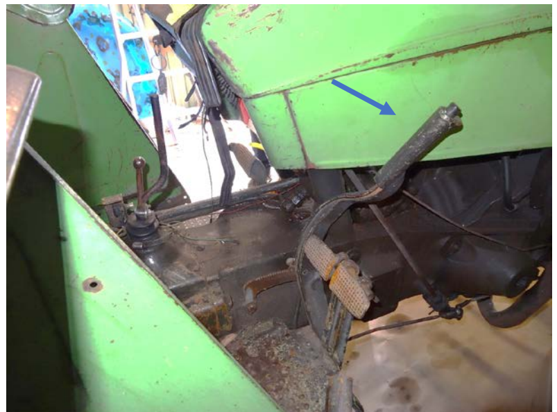
Photo 2. Arrow points to emergency brake identified by owner as non-functional
