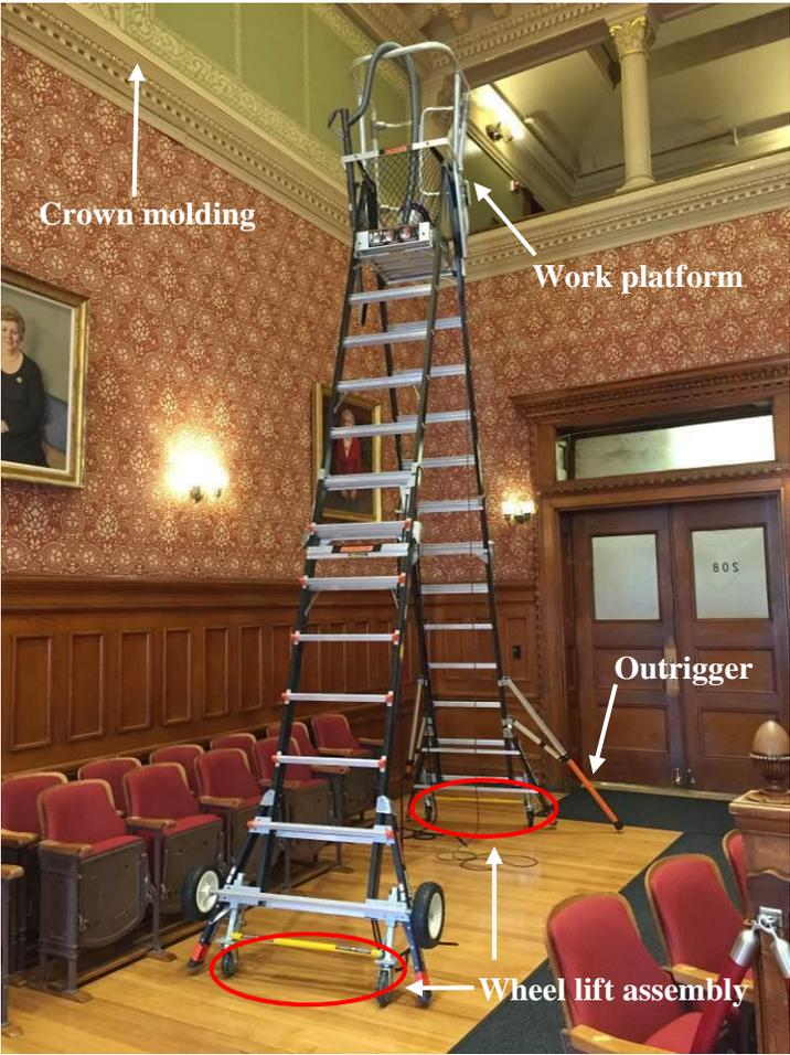
**Figure 3 – Platform ladder with one wheel lift assembly engaged and one outrigger deployed**
