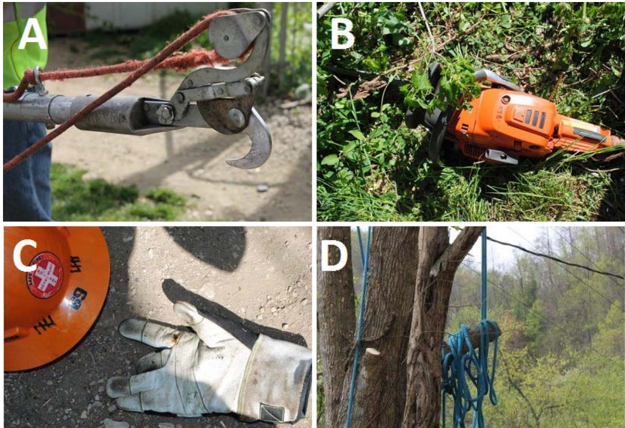
Figure 5. Insulated pruner pole (A); chainsaw (B); hard hat and leather work gloves (C); and climbing rope (D).
