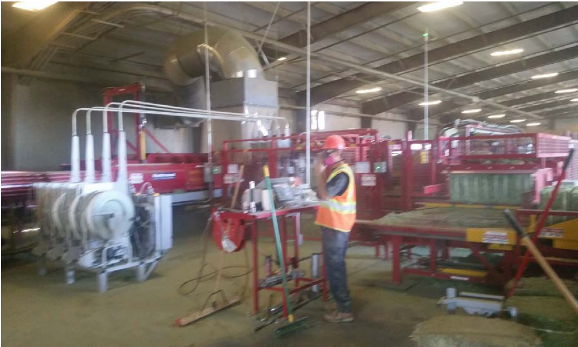
Exhibit 3. The hay baler operator's station.
