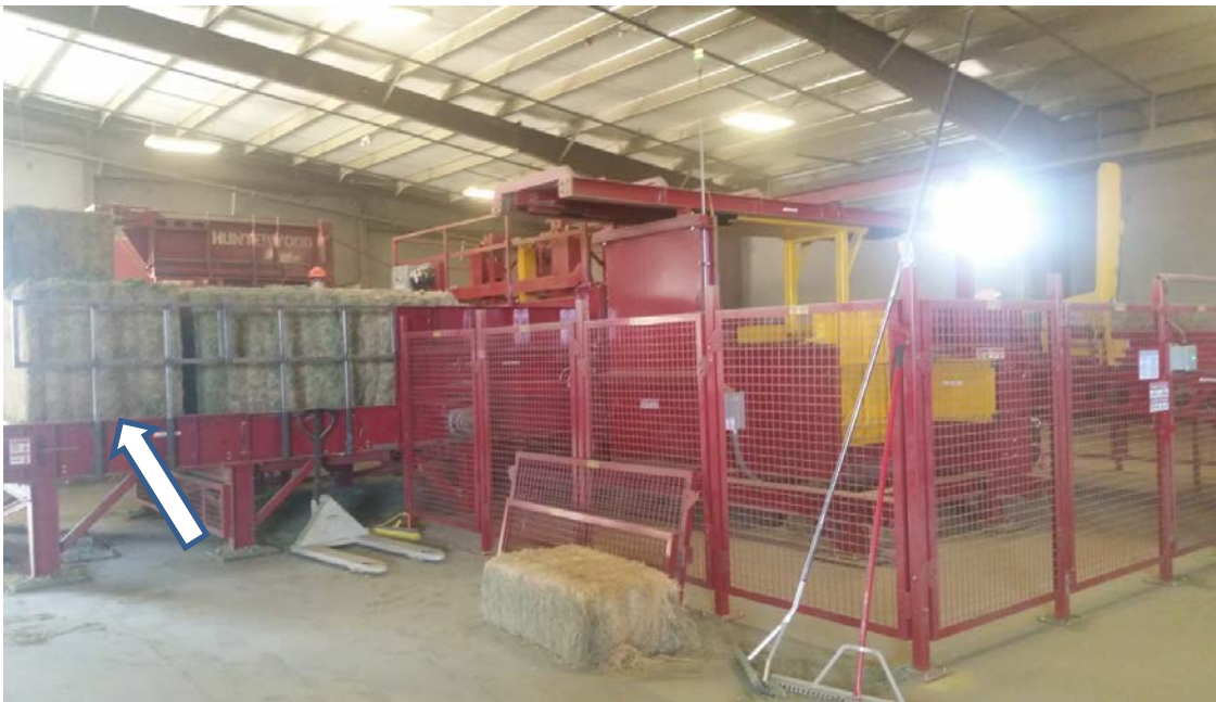
Exhibit 1. The intake portion of the hay baler.
