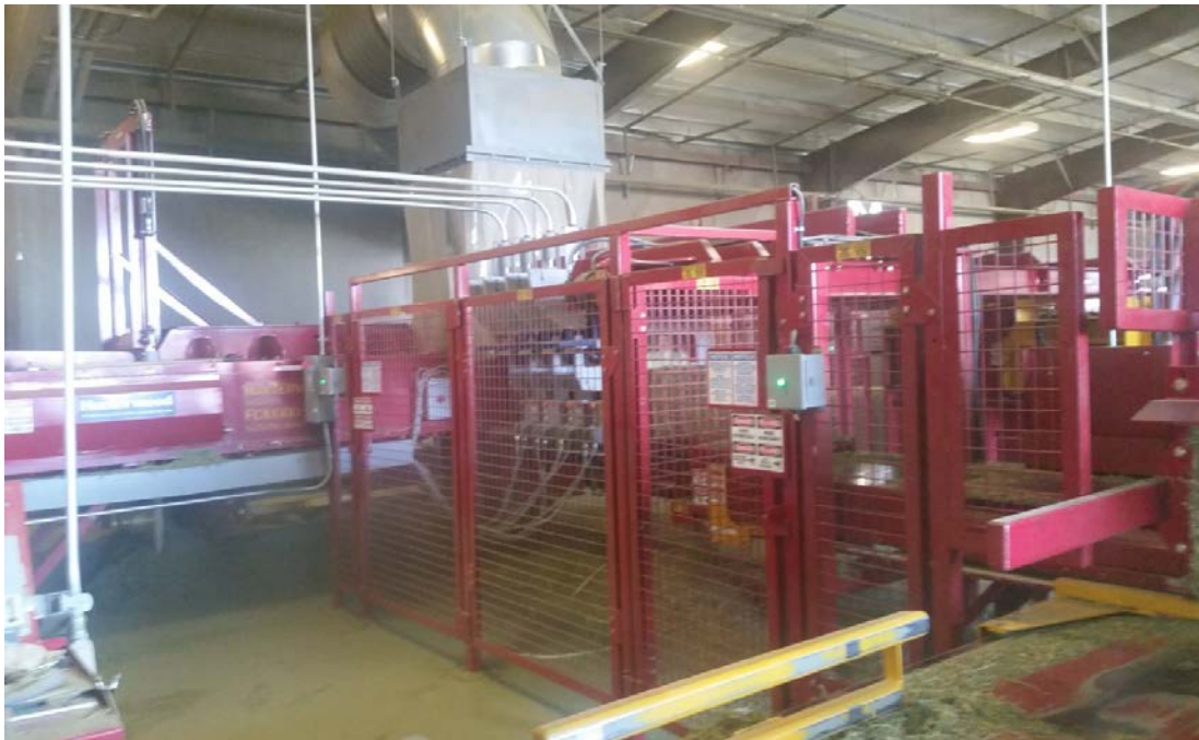
Exhibit 4. The hay baler compression, strap chamber, output scale and cutter box.
