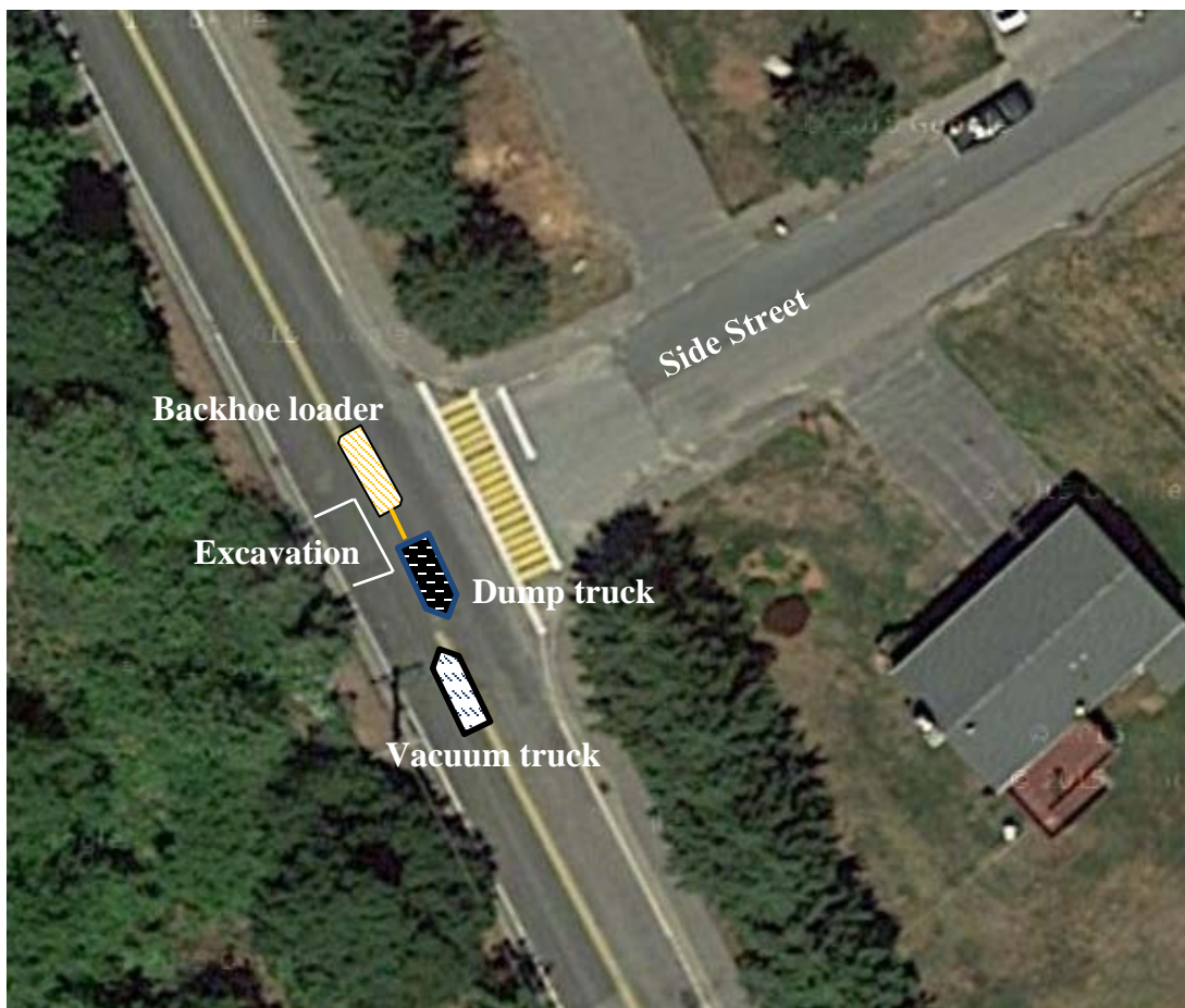
Figure 4 – Roadway view of the T-shaped intersection with outline of vehicles and excavation location
