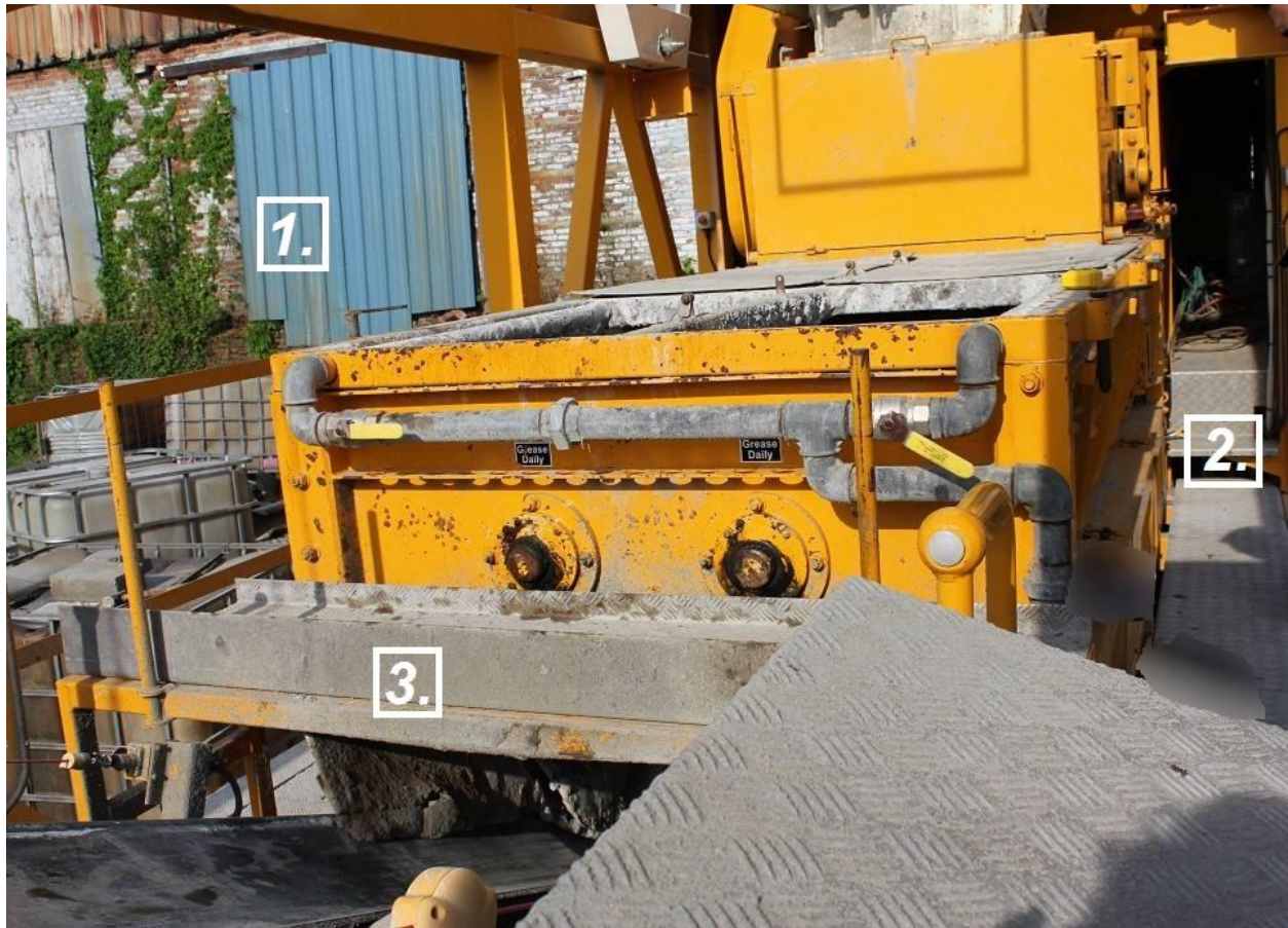
Photo 2: One walking platform on each side of the mixer, and a third elevated platform directly over the conveyor belt that connects sides 1 and 2.
