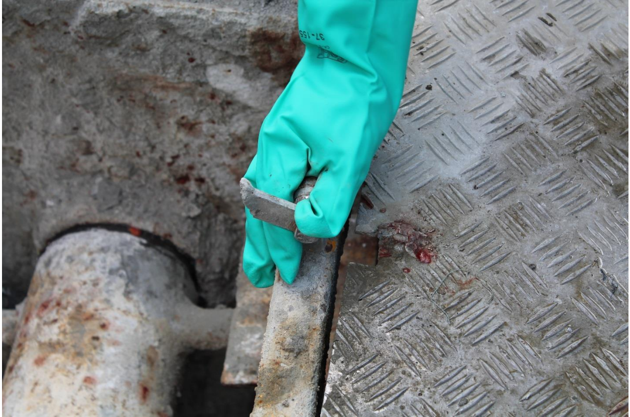
Photo 5: broken door hinge on the metal door covering the auger.
