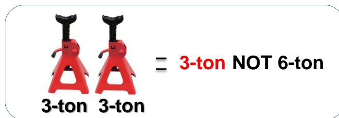
Figure 5. Rating capacity of a jack stand is established for a pair.
