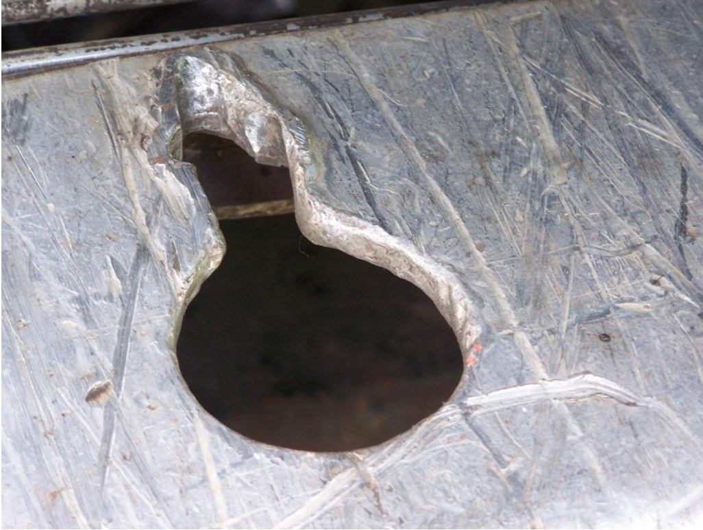
A worn securement site on the tow truck.
