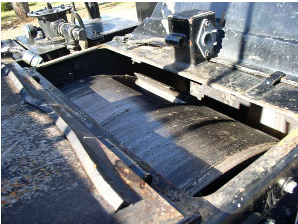
Exhibit 5. The wood chipper's drum that the rope was wrapped around.
