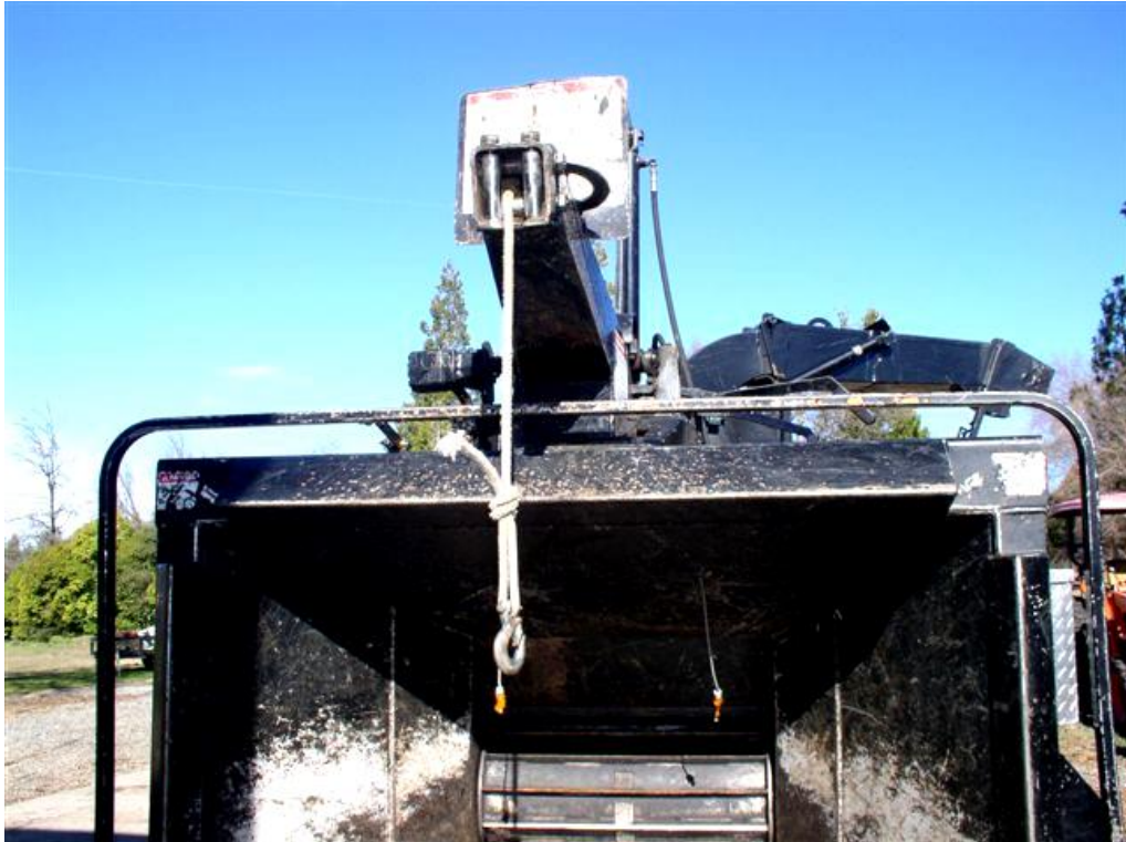
Exhibit 4. The rope winch on the wood chipper used to pull tied bundles of brush and cut branches up to the feed table.
