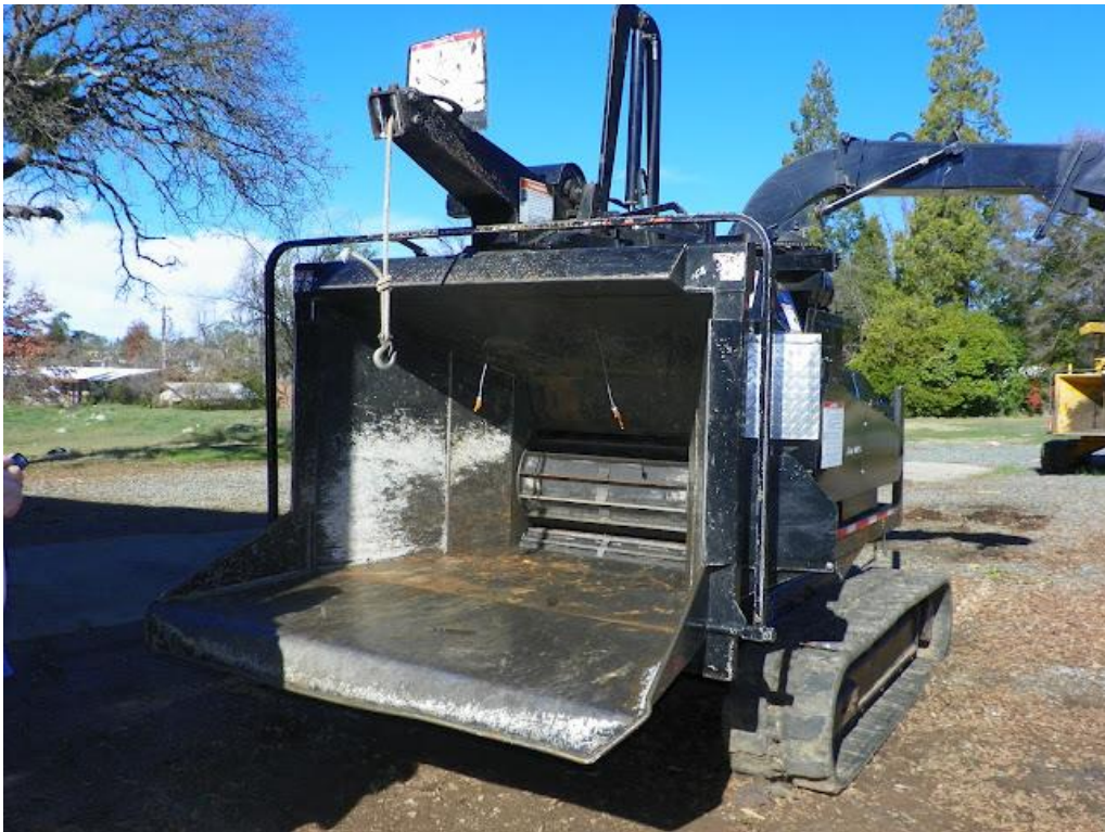
Exhibit 3. The wood chipper feed table and feed rollers.
