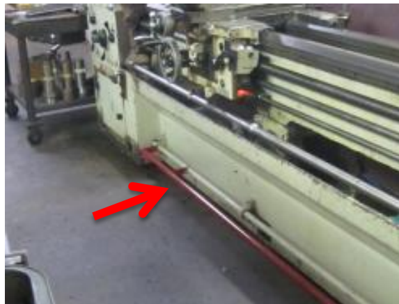
Brake bar on the engine lathe, which was painted red following the incident
