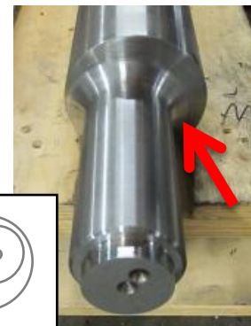
ABOVE: A finished eccentric shaft. Arrow indicates the transition of the radius of the two centers. The black and white drawing is a face schematic of the shaft end.
