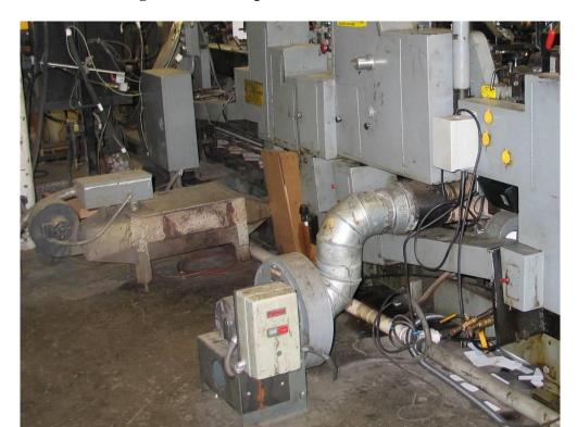
Figure 2 – Envelope machine's blower motor
