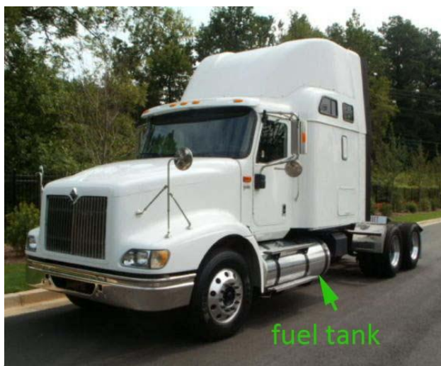
Exhibit 5. Example of 2007 International 9400I showing fuel tank location
