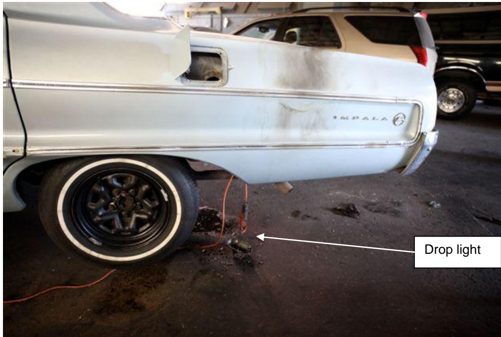
Exhibit 7. The drop light that was left hanging under the vehicle when the automotive lift was lowered.
