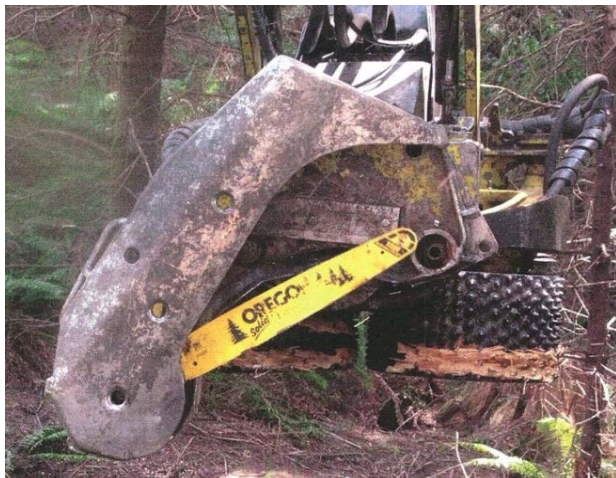
Photo 3: Timberjack 762C cutting head and Oregon roller tip 18H bar.
