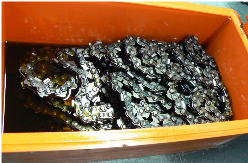
Photo10: Photo showing the inside of the orange bins with motor oil used to pre-lube chains.
