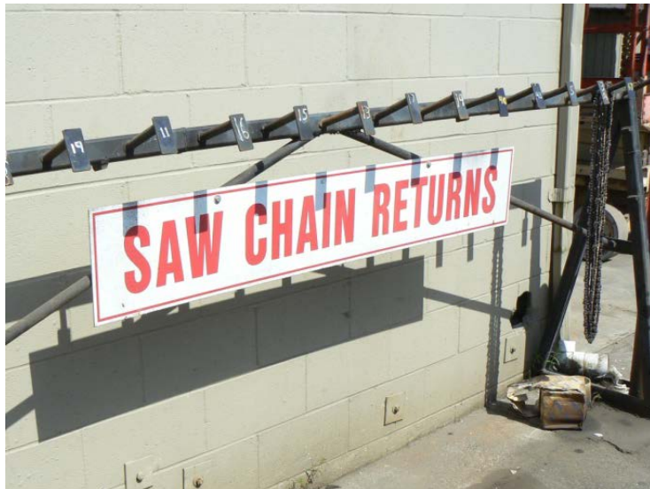
Photo 11: The numbered chains return rack used by equipment operators.
