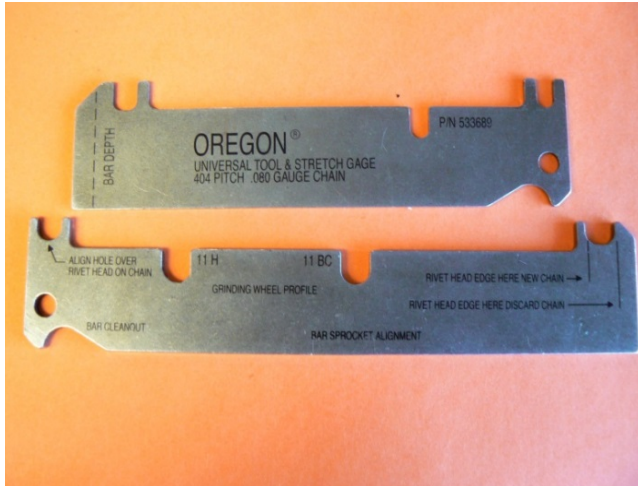
Photo 13: Tools used for inspecting chain stretch and bar depth.
