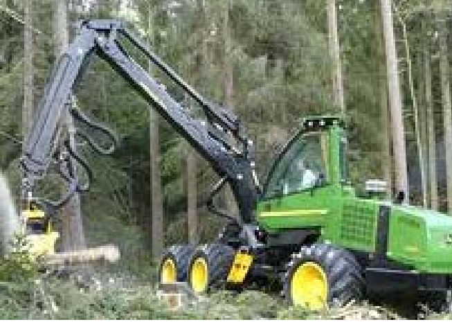
Photo 5: Photo of a harvester in the action of processing a tree with a cutting head. This particular harvester is designed so that the cab and boom with attached cutting head articulate independently. This allows the operator to position the cab so that it is not in line with the cutting bar while processing. (Not the harvester involved in the incident.)
