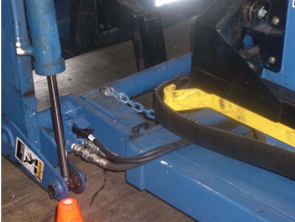
Exhibit 6. The hydraulic and electric connections.
