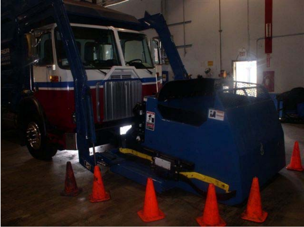
Exhibit 2. The collection bin with attached automated system
