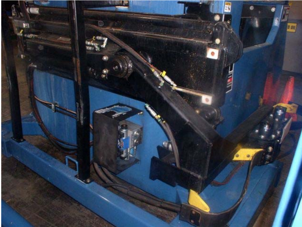
Exhibit 4. The automated systems components mounted on the rear of the collection bin.
