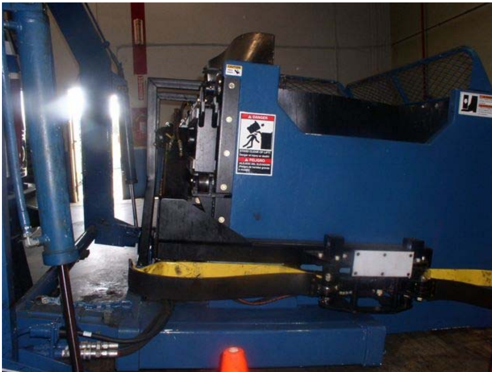
Exhibit 5. The grabbing device that extends and retracts to pick up recyclable containers.
