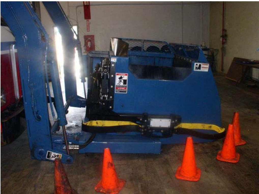
Exhibit 3. A side view of the collection bin and the automated system
