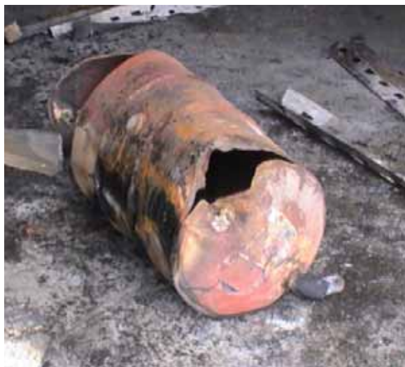
Figure 5. Waste drum after explosion.
