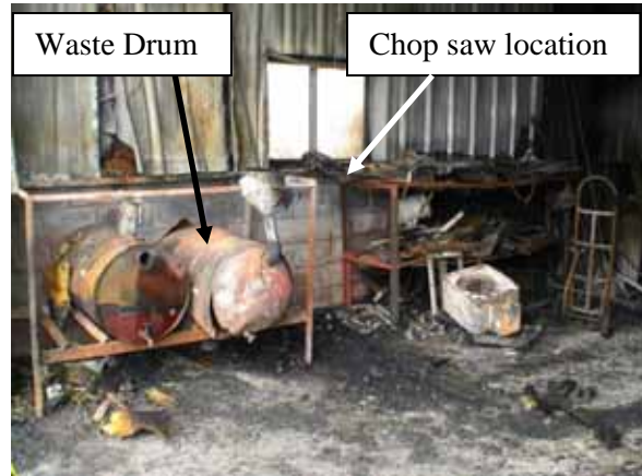
Figure 1. Position of chop saw table and drum rack with waste and motor oil drums.
