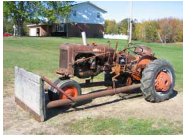
Figure 2. Incident tractor showing home-made push blade attachment
