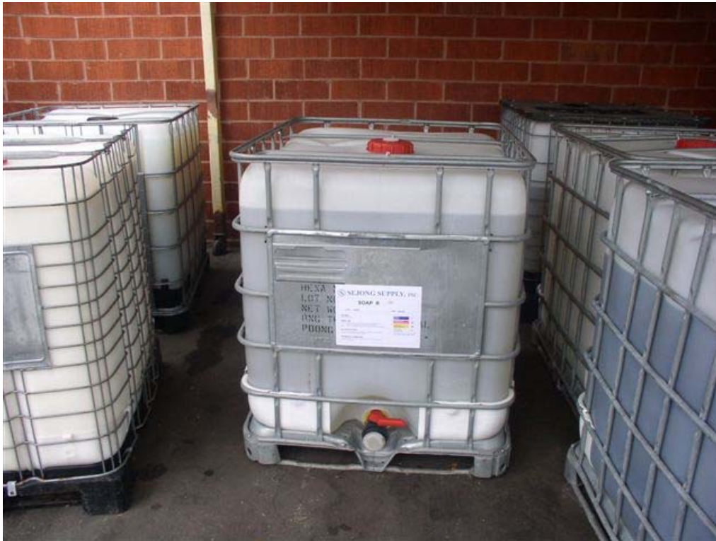
Exhibit 4. A chemical container (tote) similar to the one the victim had raised up on the forklift to transfer its contents.
