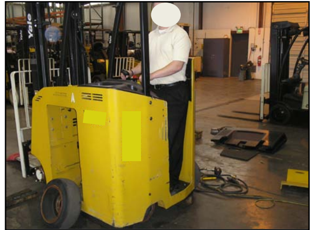
The actual forklift in this incident (with identifying images masked out) was a stand-up model for warehouse work.
