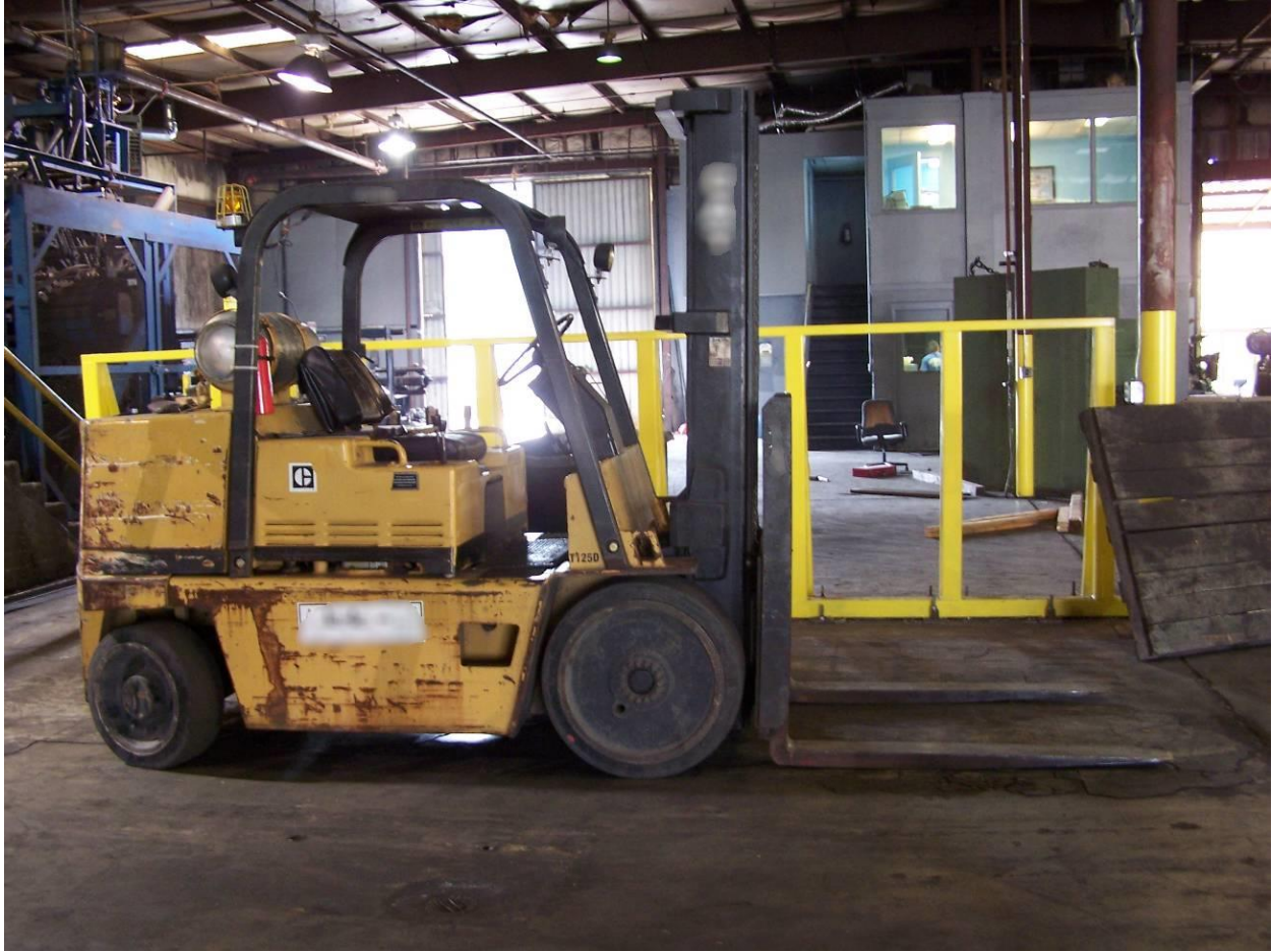
Picture of forklift used to transport steel coils. The holding area for the coils is on the other side of the yellow barrier.
