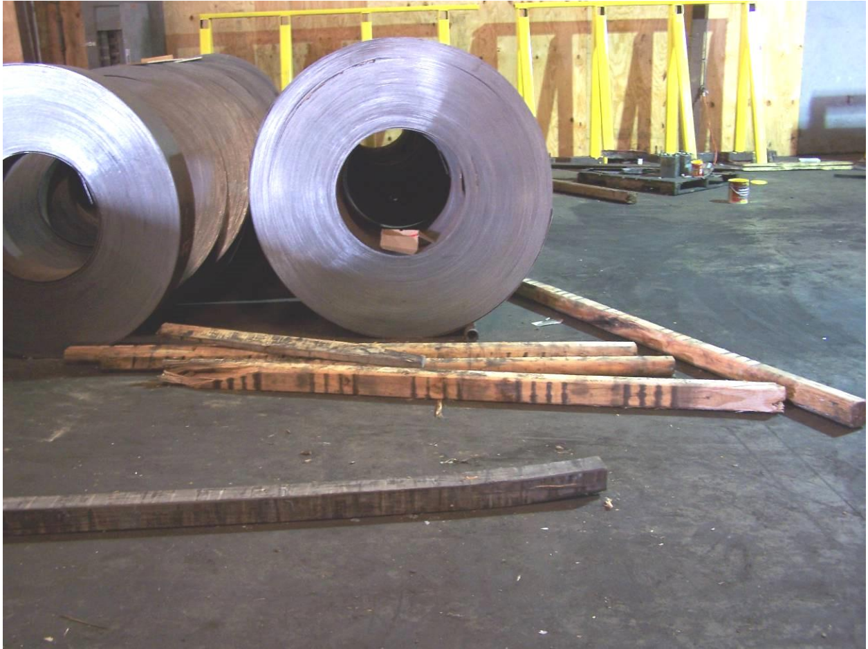
Picture of coils of slitted steel in the storage area waiting to be transported to the holding area before being taken to the pipe mill.
