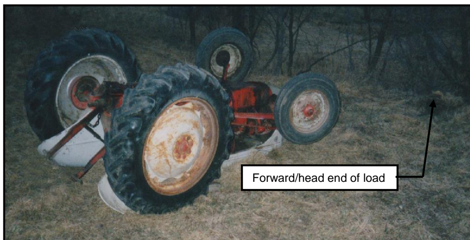
Photo 1 – Tractor shown overturned to rear toward load it was towing with a cable.
