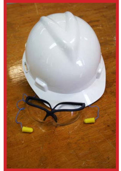
PPE such as a hardhat, safety glasses, and ear plugs aid in protecting worker health and safety
