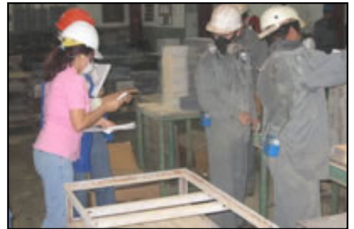
A Ministry of Health of El Salvador staff member checks workers' personal air monitors during the Ministry's lead exposure assessment in Salvadoran battery recycling/manufacturing plant. Photo courtesy of Aaron Sussell.
