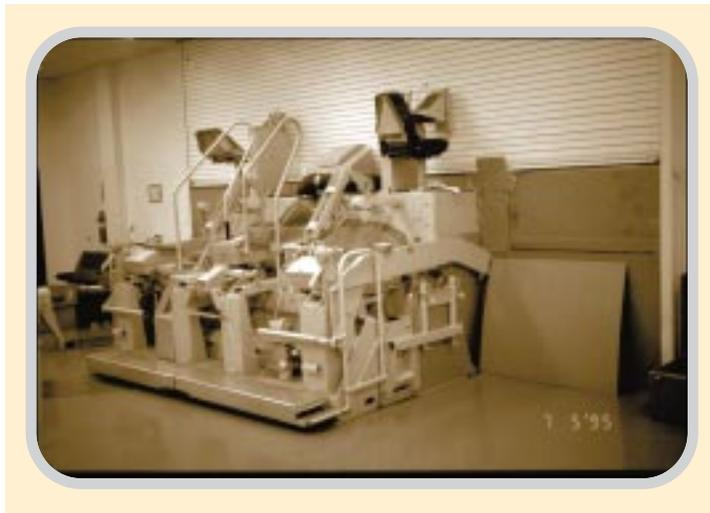
Figure A-1. Test area rear half of paver isolated from front half of paver.
