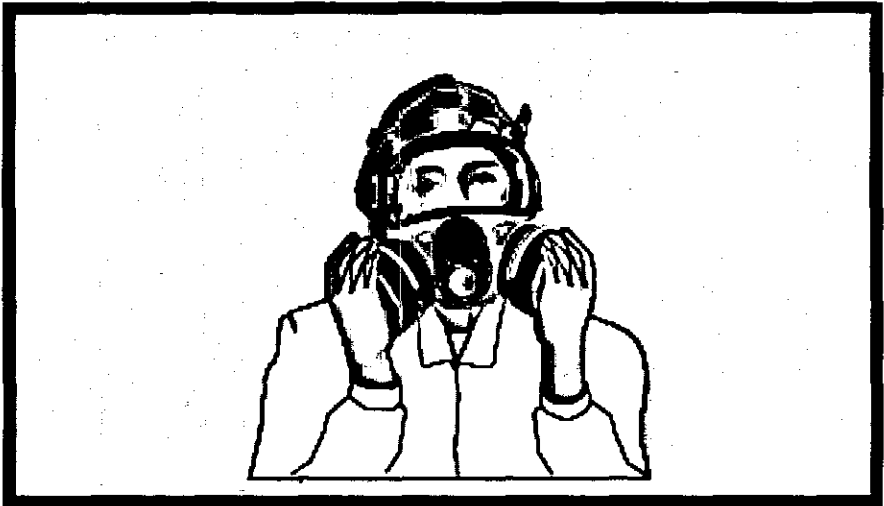
Fit Check: worker covering inlet and inhaling.
