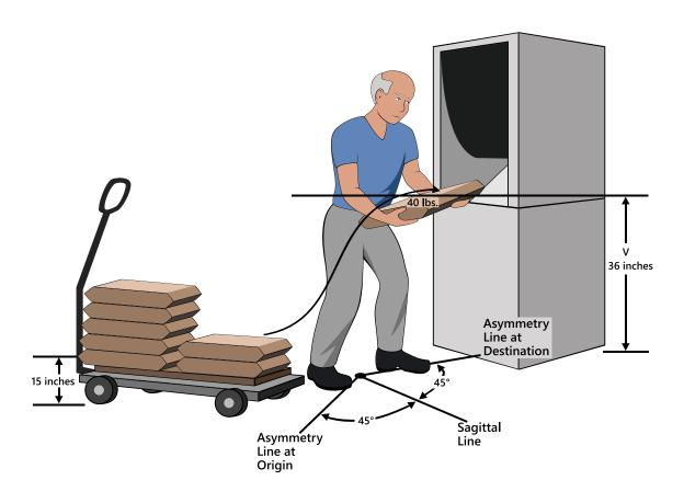
Figure 11: Loading Bags Into Hopper, Example 3
