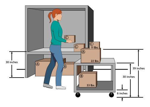
Figure 27: Warehouse Order Filling, Example 10
