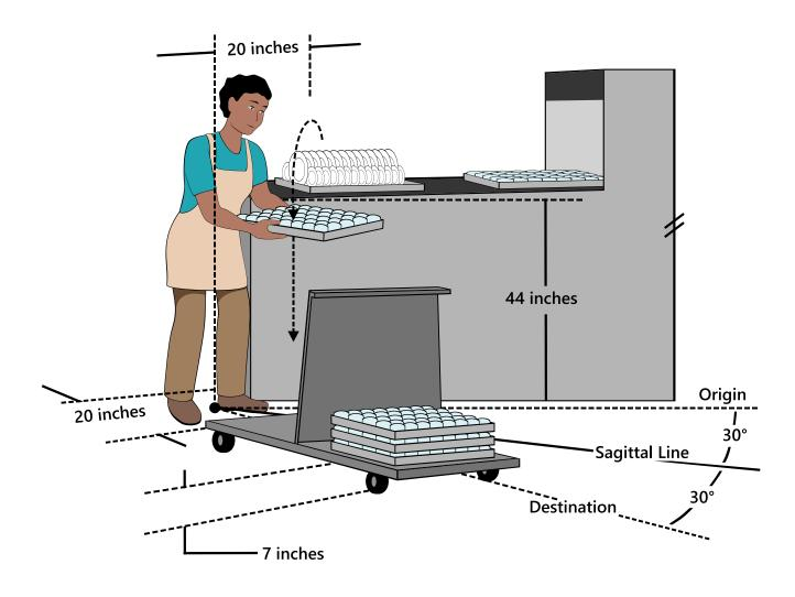
Figure 15: Dishwashing Machine Unloading, Example 5
