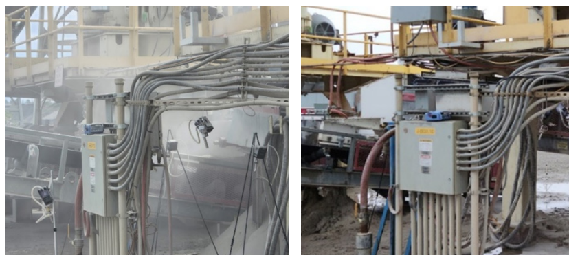
Figure 3. Before and after photos show the 93% decrease in respirable dust in air. Photo by NIOSH.
