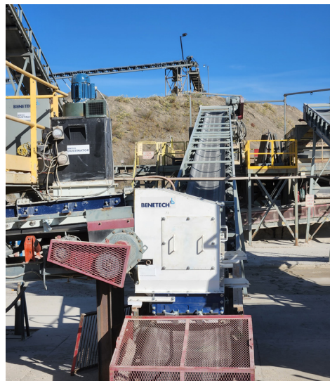
Figure 1. Prototype hybrid dust control system retrofitted onto a crusher-conveyor system at a mine site. Photo by NIOSH.
