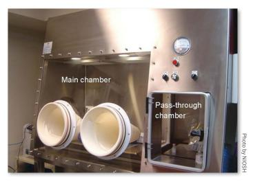
**Figure 3.** Compounding aseptic containment isolator (CACI) cabinet.
