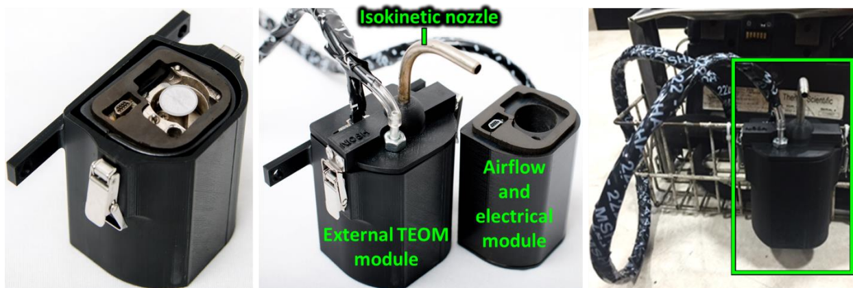
Figure 6.3. External sampling housing with the TEOM unit inserted (left). The external TEOM module with isokinetic nozzle is connected to airflow and electrical module (center), which inserts into the PDM body. A modified TEOM module is mounted on a sampling basket (right).
