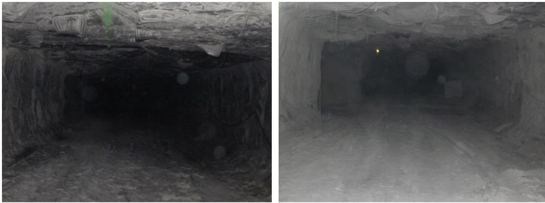
Figure 6.5. Return entry after a cut without (left) and with flooded bed scrubber operating (right) illustrating difference in float coal dust deposition.
