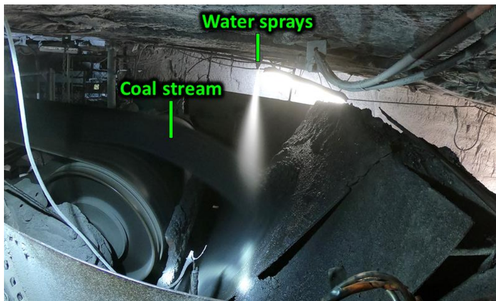
Figure 6.8. Water sprays directed at top of coal stream being discharged from belt.
