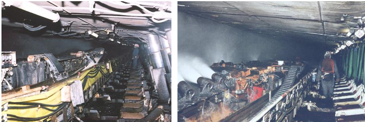
Figure 3.29. Photos illustrating dust confined near face as seen from the tailgate shearer operator's position on a tail-to-head pass (left) and the headgate shearer operator's position on a head-to-tail pass (right).
