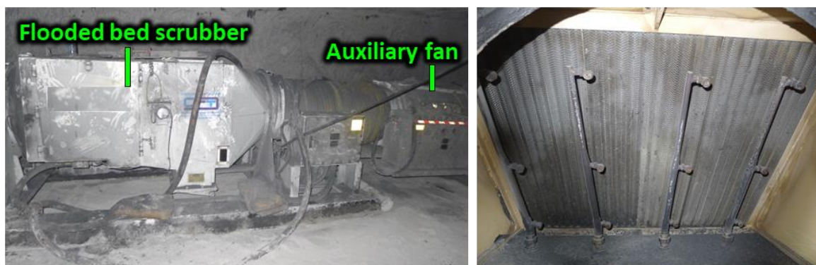
Figure 6.4. Flooded bed scrubber unit (left) and 12 water sprays used to wet filter panel (right).
