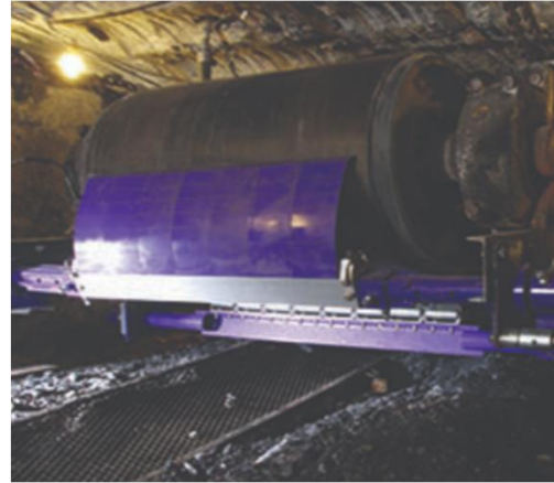
Figure 3.11. Typical locations of primary and secondary belt scrapers (left) and a photo of a primary belt scraper installed (right).
