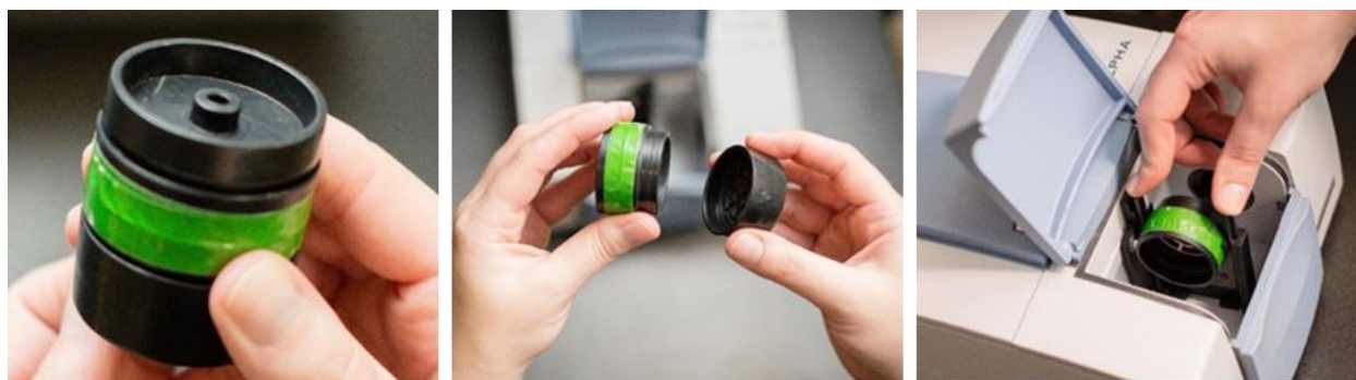
Figure 2.7. Four-piece cassette (left) with filter contained within two center sections (center) and being loaded into an FTIR instrument cradle (right).
