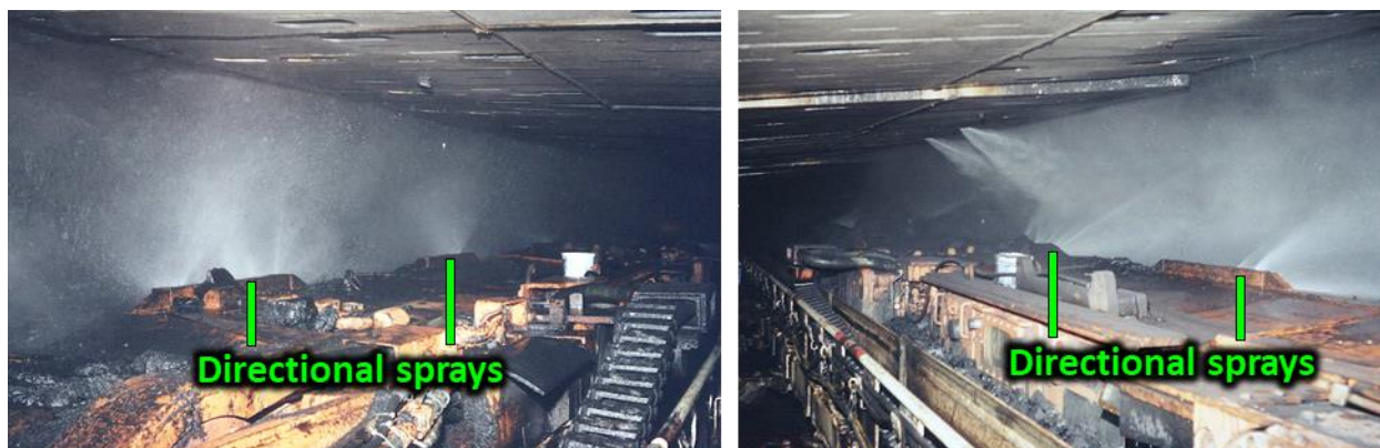
Figure 3.24. Directional spray manifolds mounted on face side of shearer body as viewed from the headgate (left) and tailgate (right) sides of the shearer.
