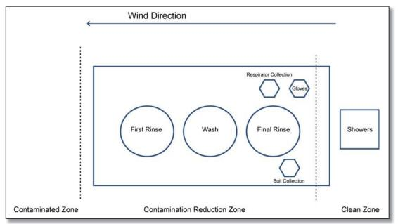
Figure 8-1. Simplified Decontamination Station.
