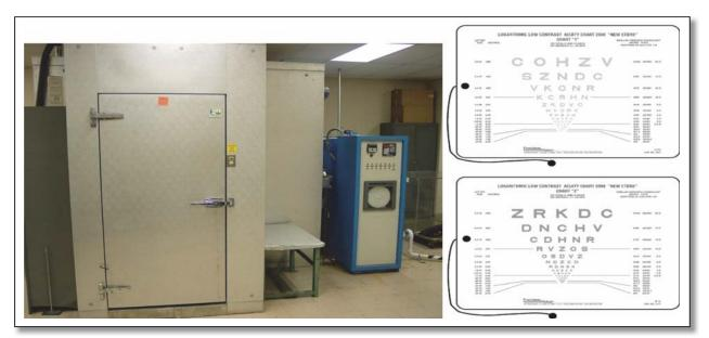
Figure 2-19. Low Temperature/Fogging Test
