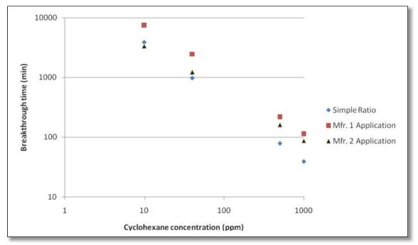
Figure 4-2. Estimated Breakthrough Times for Cyclohexane
