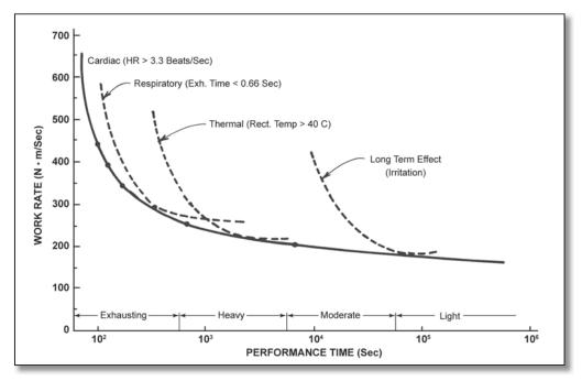
**Figure 7-4.** Schematic Representation of Performance Time While Exercising and Wearing a Protective Mask [Johnson and Cummings 1975]
