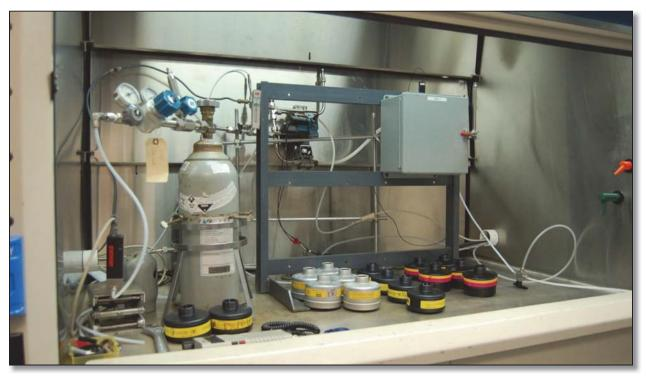
Figure 2-8. NIOSH Service Life Test Chamber
