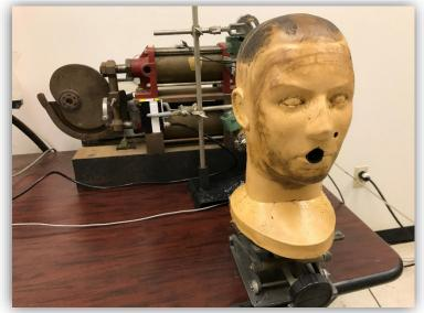
Figure 2-15. NIOSH CO<sub>2</sub> Test Apparatus
