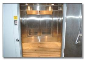
**Figure 2-13.** Inside view of NIOSH Environmental Conditioning Chamber
