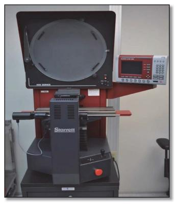
Figure 2-16. NIOSH Optical Thread Comparator
