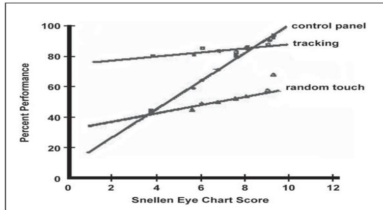
**Figure 7-3.** Performance for several tasks as visual acuity varies while wearing respirators. The Snellen eye chart denotes better vision for higher line numbers. Control panel recognition and performance ability is particularly sensitive to visual acuity.
