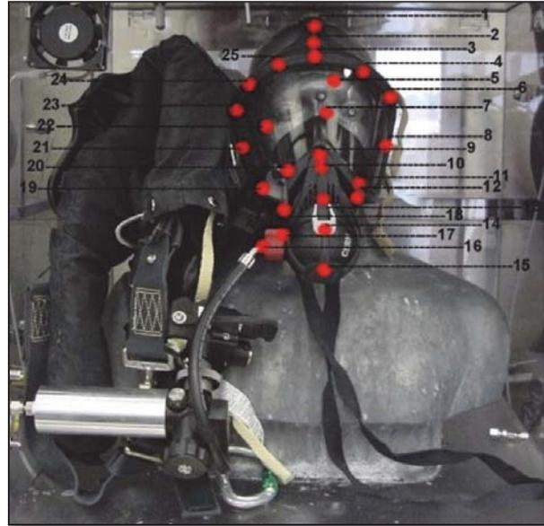
**Figure 2-6.** SCBA in Live Agent Test Chamber
