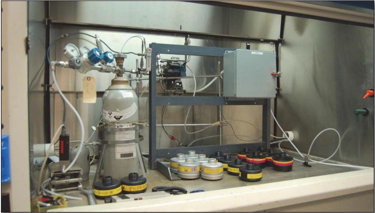
Figure 2-8. NIOSH Service Life Test Chamber
