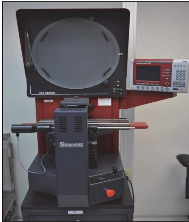
**Figure 2-16.** NIOSH Optical Thread Comparator
