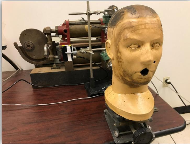
**Figure 2-15.** NIOSH CO<sub>2</sub> Test Apparatus
